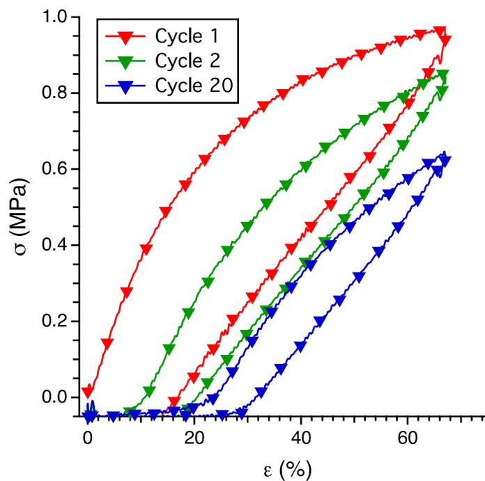
**Figure S24.** Hysteresis test of LCD77L (34.2, 0.30) conducted at a constant crosshead velocity of  $110 \text{ mm min}^{-1}$  and strain of 67%. The data shown are for cycles 1, 2, and 20 of a 20-cycle experiment with no recovery between cycles. The energy loss data for this test are 55% and 38% for the first and second cycle, respectively. The recovery between first and second cycle is 65%, between the first and twentieth cycle recovery is 33%.
