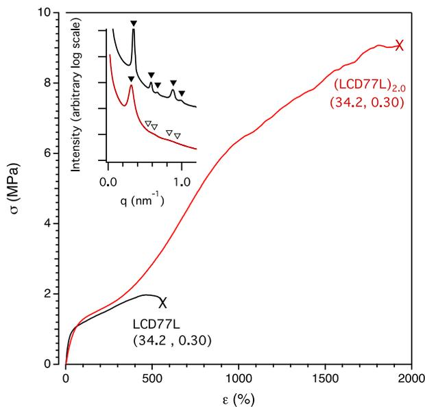
**Figure S22.** Representative examples of room temperature uniaxial extension of a LCD77L triblock and corresponding (LCD77L)<sub>n</sub> multiblock. Experiments were conducted with constant crosshead velocity of 50 mm min<sup>-1</sup>. For each sample, average and standard deviation of a minimum of 5 specimens is reported in Table S11. The graph inset displays room temperature SAXS data of compression molded LCD69L elastomers prior to uniaxial extension test.
