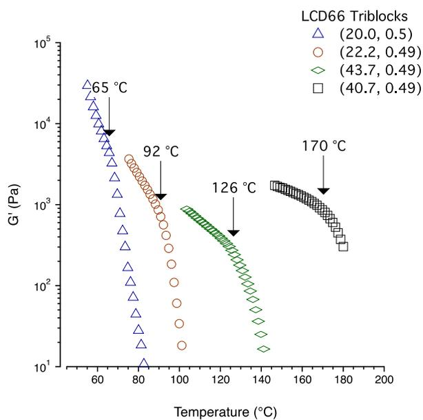
**Figure S5.** Isochronal temperature ramp data on heating ( $1 \text{ rad s}^{-1}$ ,  $1^\circ\text{C min}^{-1}$ , 1% strain) on LCDL triblock copolymers LCD65L (20.0, 0.50), LCD66L (22.2, 0.5), LCD67L (43.7, 0.49), LCD63L (40.7, 0.49).
