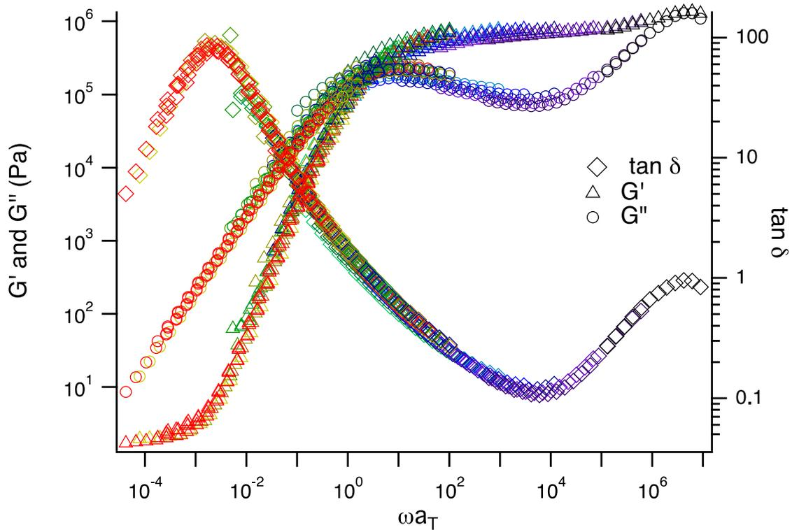
**Figure S14.** PCD63 Master curve created using isothermal frequency sweeps (100 to 0.1 rad sec<sup>-1</sup>) data were acquired from 180 °C to -30 °C. The reference temperature used is 25 °C. The shift factors were obtained by shifting  $\tan \delta$  and applied to  $G'$  and  $G''$ . No vertical shifts were applied. Shift factors and fit to the WLF equation are shown in S15 and S16.
