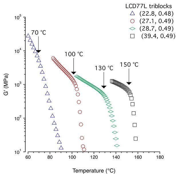
**Figure S6.** Isochronal temperature ramp data on heating ( $1 \text{ rad s}^{-1}$ ,  $1^\circ\text{C min}^{-1}$ , 1% strain) for LCDL triblock copolymers LCD78L (22.8, 0.48), LCD77L (27.1, 0.49), LCV76L (28.7, 0.49), LCV76L (39.4, 0.49).
