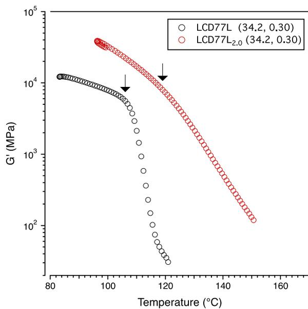
**Figure S13.** Isochronal temperature ramp data on heating ( $1 \text{ rad s}^{-1}$ ,  $1^{\circ}\text{C min}^{-1}$ , 1% strain) for LCD77L (34.2, 0.3). Isochronal temperature ramp data on heating ( $0.1 \text{ rad s}^{-1}$ ,  $0.2^{\circ}\text{C min}^{-1}$ , 1% strain) for multiblock (LCD77L)<sub>2.0</sub> (34.2, 0.3).
