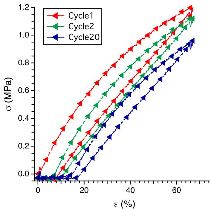
**Figure S25.** Hysteresis tests of  $(\text{LCD77L})_{2.0}$  (34.2, 0.30) conducted at a constant crosshead velocity of  $110 \text{ mm min}^{-1}$  and strain of 67%. The data shown are for cycles 1, 2, and 20 of a 20-cycle experiment with no recovery between cycles. The energy loss data for this test are 31% and 20% for the first and second cycle, respectively. The recovery between the first and second is 71%, between the first and twentieth cycle recovery is 60%.
