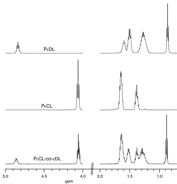
**Figure S1.**  $^1\text{H}$  NMR spectra of poly( $\epsilon$ -decalactone), poly( $\epsilon$ -caprolactone), and poly( $\epsilon$ -decalactone-*co*-caprolactone) showing the resonances used to determine copolymer composition.
