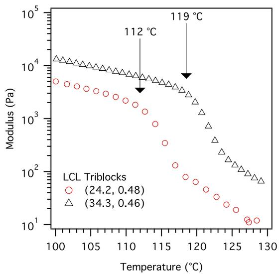
**Figure S9.** Isochronal temperature ramp data on heating ( $1 \text{ rad s}^{-1}$ ,  $1^{\circ}\text{C min}^{-1}$ , 1% strain) for LCL (24.2, 0.48) and LCL (34.3, 0.46). The data for LCL (34.3, 0.46) have been shifted vertically for clarity.
