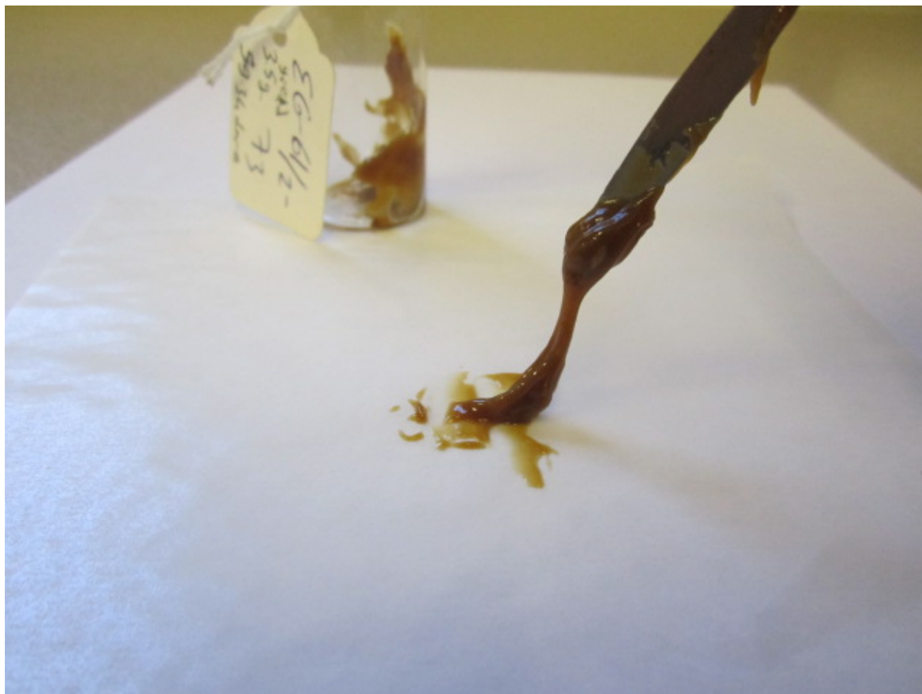
Figure S166. Photograph of mostly waxy, amorphous, oligomeric material (Table S1 entry 8) obtained according to the trioxane/CO copolymerization method described by G. Cevidalli, M. Ragazzini, and M. Modena, U.S. Patent 3,673,156, 1972 .
