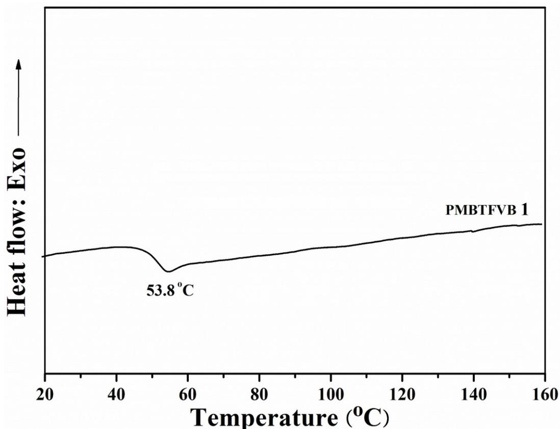
**Figure S3.** Third heating DSC scan (in N<sub>2</sub>) of PMBTFVB **1** with a heating rate of 10°C/min.
