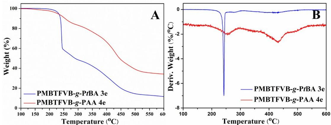
**Figure S2.** TGA (A) and DTG (B) curves (in N<sub>2</sub>) of PMBTFVB-g-PtBA **3e** and PMBTFVB-g-PAA **4e** graft copolymer with a heating rate of 10°C/min.
