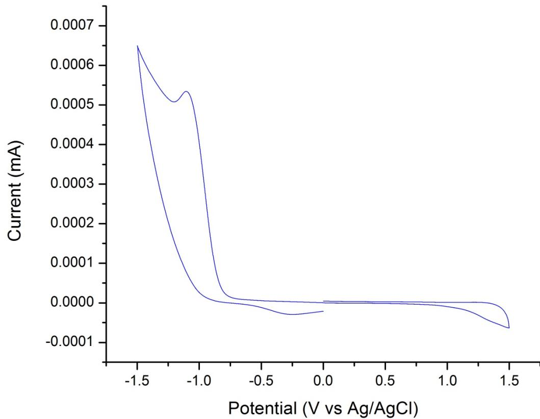
Figure S13: Cyclic Voltammogram of PAAC
