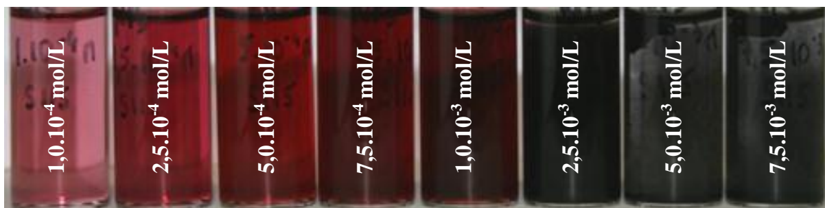
Figure SI 14. Au NPs solutions formed at different \text{HAuCl}_4 concentrations 10 minutes from the addition of \text{NaBH}_4 to \text{HAuCl}_4 ( [\text{HAuCl}_4]/[\text{NaBH}_4] = 1 ).
