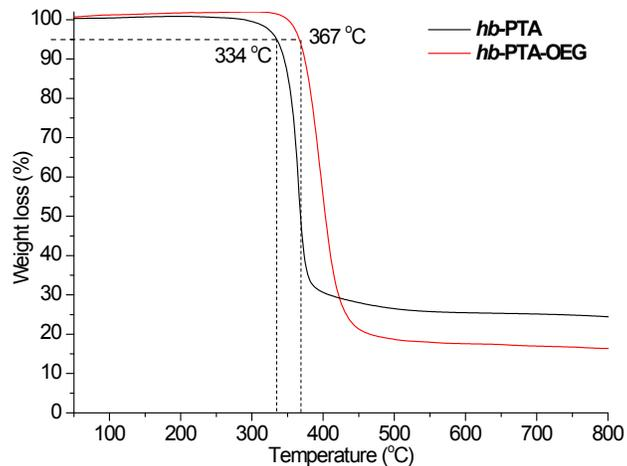
**Fig. S2** TGA curves of (a) *hb-PTA* and (b) *hb-PTA-OEG*.
