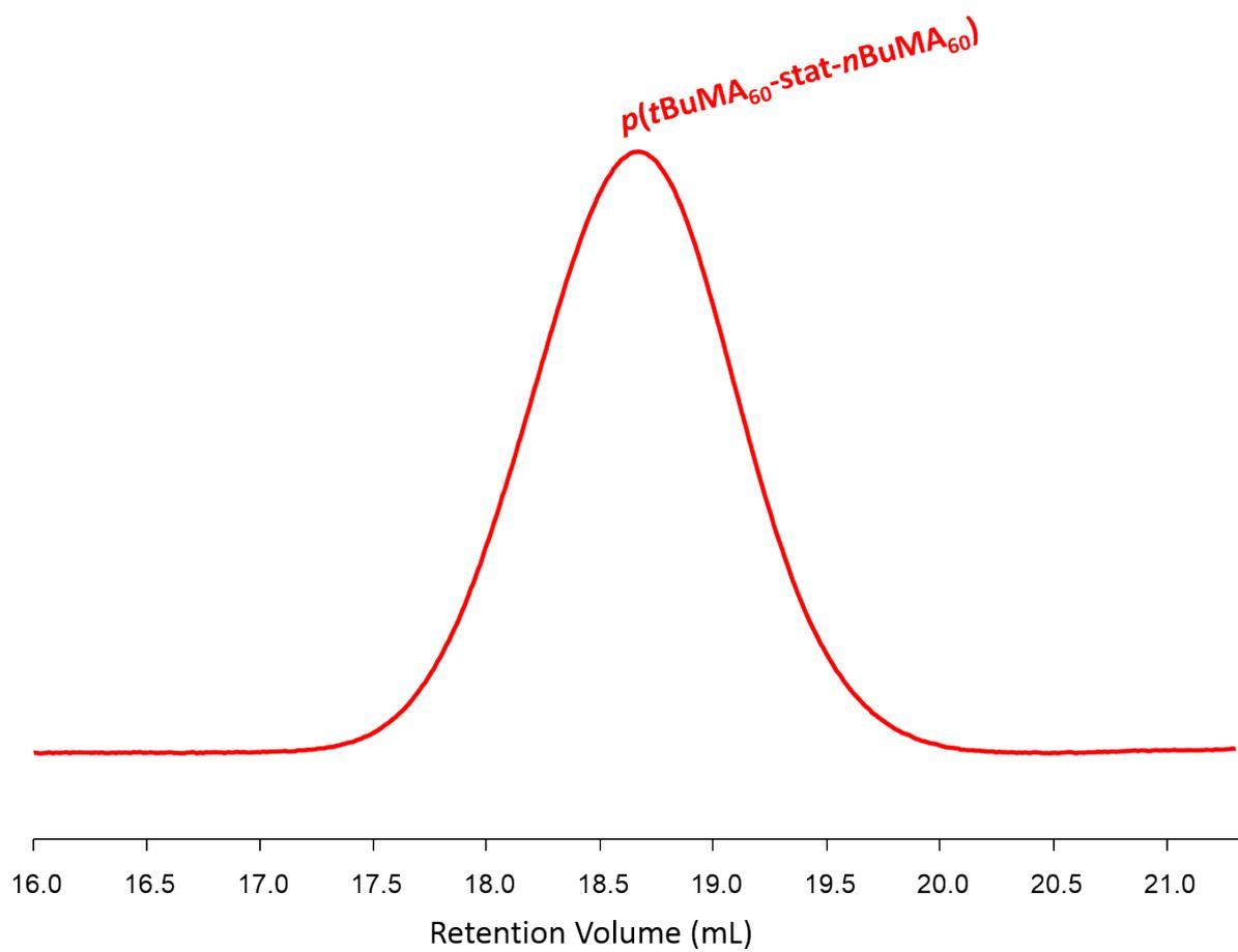
**Figure S23** SEC chromatogram (RI) of the  $p(t\text{BuMA}_{60}\text{-stat-}n\text{BuMA}_{60})$  statistical copolymer produced via methanolic Cu-catalysed ATRP of  $t\text{BuMA}$  and  $n\text{BuMA}$  at 60 °C, targeting  $\text{DP}_n = 60$  monomer units for each comonomer. Analysis performed by triple detection SEC with a mobile phase of THF (+ 2 v/v % TEA) at 1 mL/min, 35 °C.
