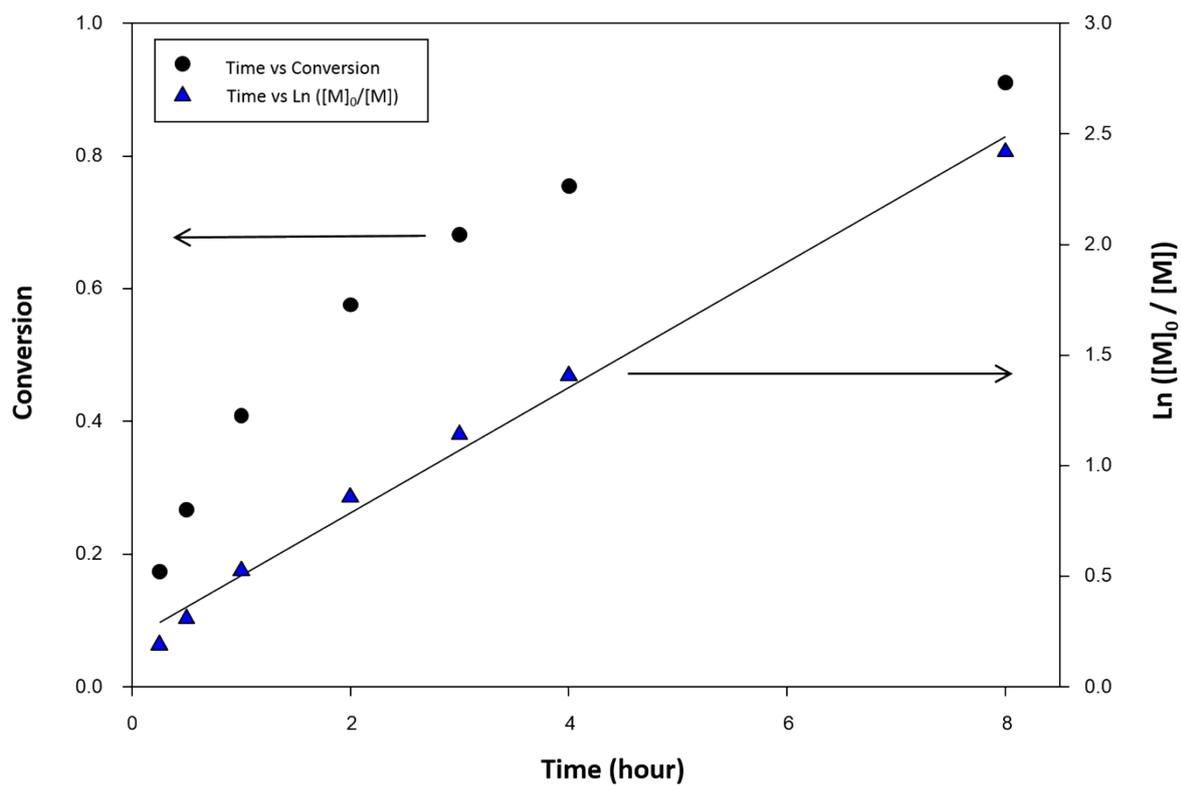
**Figure S16;** Kinetic studies of  $p(\text{PEG}_{113}\text{-}b\text{-}n\text{BuMA}_{80})$  synthesis *via* Cu-Catalysed ATRP in anhydrous methanol at  $60\text{ }^\circ\text{C}$  showing conversion and semilogarithmic plots *vs.* time.
