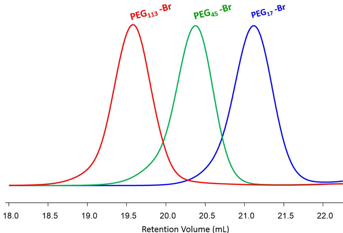
**Figure S9** Overlaid SEC (RI) chromatograms of the monofunctional PEG<sub>17</sub>-Br, PEG<sub>45</sub>-Br, and PEG<sub>113</sub>-Br macroinitiators. Analysis performed by triple detection SEC with a mobile phase of DMF (+ 0.01M LiBr) at 1mL/min, 60 °C.
