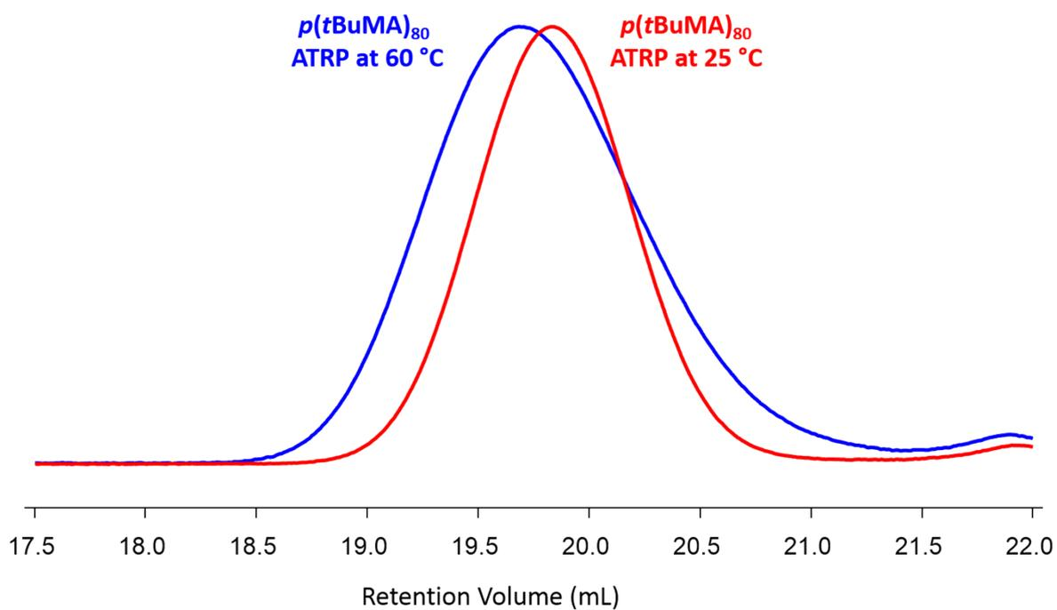
**Figure S6** Overlaid SEC chromatograms (RI) of linear homopolymers produced using methanolic Cu-catalysed ATRP of *t*BuMA at 25 °C (red) and 60 °C (blue), targeting  $DP_n = 80$  monomer units. Analysis performed by triple detection SEC with a mobile phase of THF (+ 2 v/v % TEA) at 1 mL/min, 35 °C.
