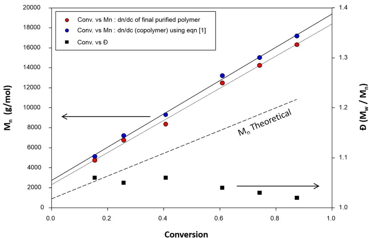
**Figure S12** Kinetic studies of  $p(\text{PEG}_{17}\text{-}b\text{-}n\text{BuMA}_{80})$  synthesis *via* Cu-Catalysed ATRP in anhydrous methanol at 60 °C showing the evolution of  $M_n$  and dispersity with conversion.
