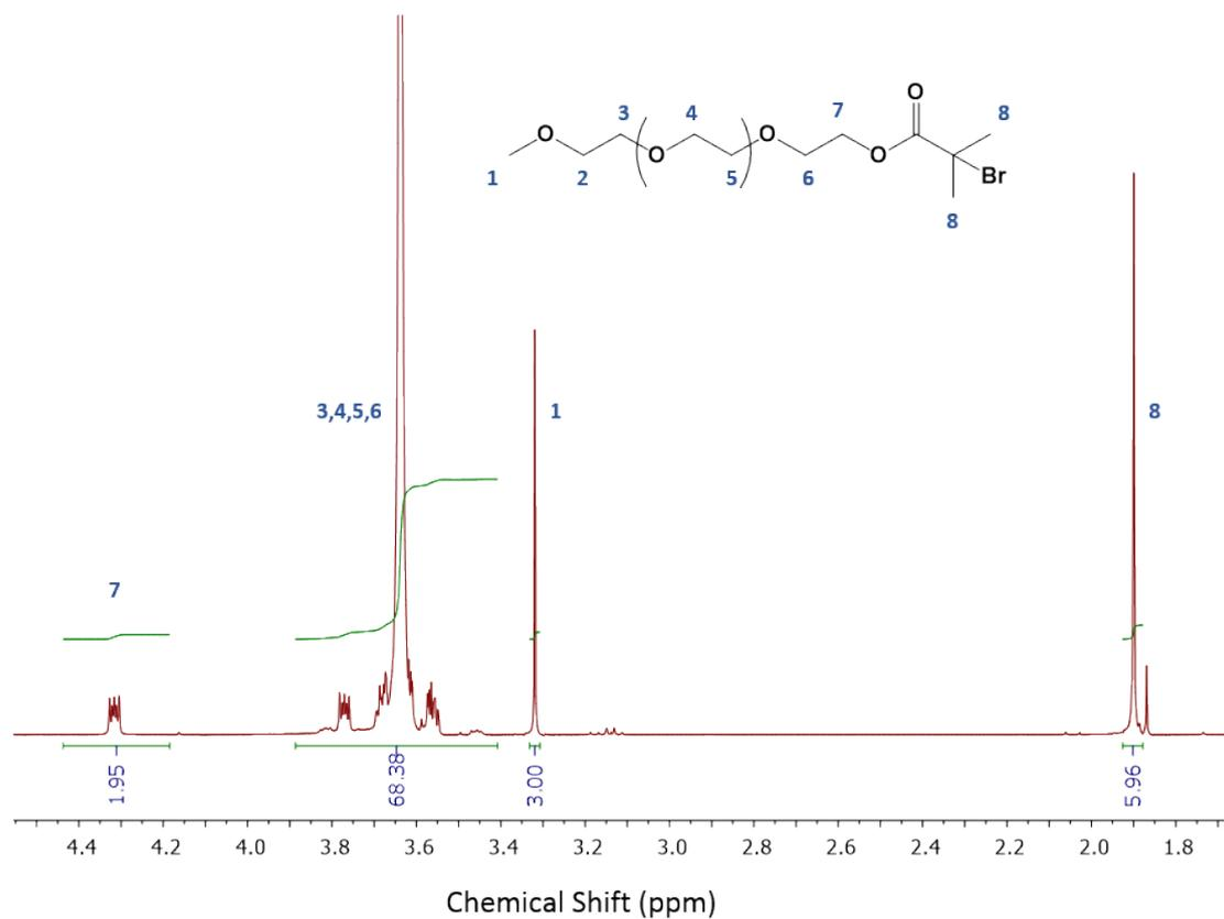
**Figure S7**  $^1\text{H-NMR}$  ( $\text{D}_2\text{O}$ ) spectrum of  $\text{PEG}_{17}\text{Br}$  macroinitiator.
