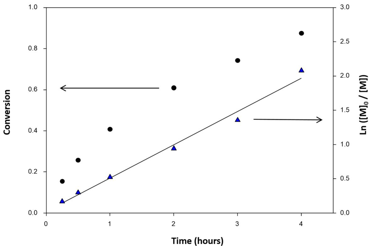
**Figure S11** Kinetic studies of  $p(\text{PEG}_{17}\text{-}b\text{-}n\text{BuMA}_{80})$  synthesis *via* Cu-Catalysed ATRP in anhydrous methanol at 60 °C showing conversion and semilogarithmic plots vs. time.
