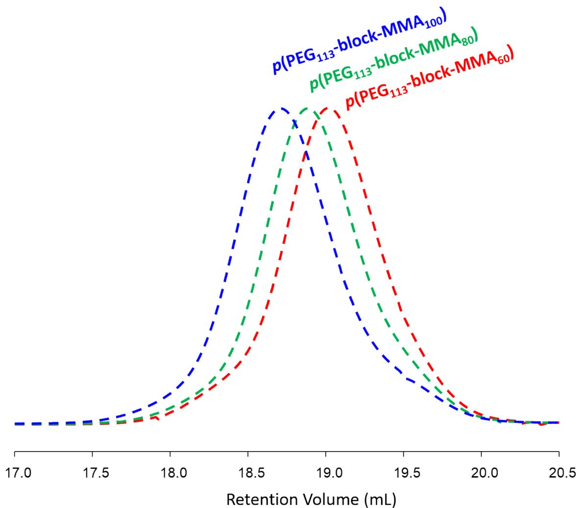
**Figure S18** Overlaid SEC chromatograms (RI) of  $p(\text{PEG}_{113}\text{-}b\text{-MMA}_x)$  A-B block copolymers produced *via* methanolic Cu-catalysed ATRP of MMA at 60 °C using  $\text{PEG}_{113}\text{-Br}$  macroinitiator across the targeted  $\text{DP}_n = 60\text{-}100$  monomer units. Analysis performed by triple detection SEC with a mobile phase of DMF (+ 0.01M LiBr) at 1 mL/min, 60 °C.
