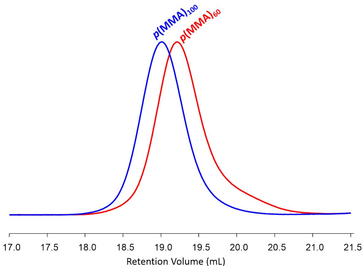
**Figure S5** Overlaid SEC chromatograms (RI) of linear homopolymers produced using methanolic Cu-catalysed ATRP of MMA at 60 °C, targeting  $DP_n = 60$  and 100 monomer units. Analysis performed by triple detection SEC with a mobile phase of THF (+ 2 v/v % TEA) at 1 mL/min, 35 °C.
