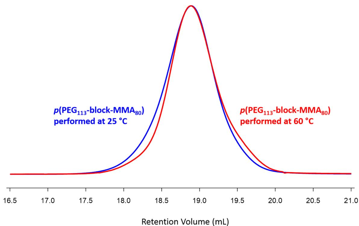
**Figure S21** Overlaid SEC chromatograms (RI) of  $p(\text{PEG}_{113}\text{-}b\text{-MMA}_{80})$  A-B block copolymers produced *via* methanolic Cu-catalysed ATRP of MMA at 25 °C (blue trace) and 60 °C (red trace), targeting  $\text{DP}_n = 80$  monomer units and using  $\text{PEG}_{113}\text{-Br}$  macroinitiator. Analysis performed by triple detection SEC with a mobile phase of DMF (+ 0.01M LiBr) at 1 mL/min, 60 °C.
