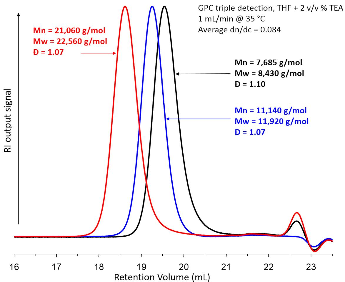
**Figure S4** Overlaid SEC chromatograms (RI) of linear homopolymers produced using methanolic RAFT of MMA at 60 °C across the targeted  $DP_n = 60$ -200 monomer units. Analysis performed by triple detection SEC with a mobile phase of THF (+ 2 v/v % TEA) at 1 mL/min, 35 °C.
