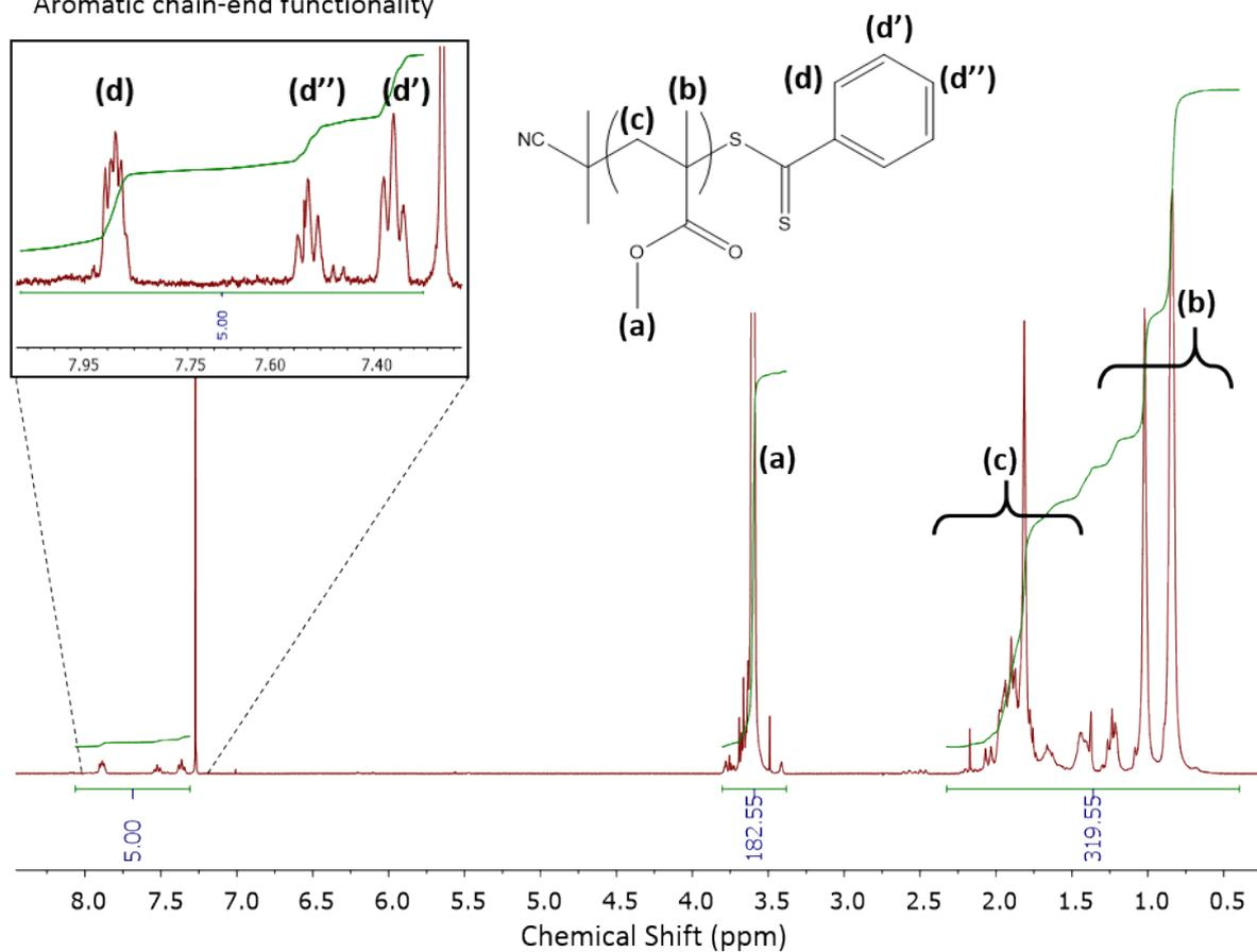
**Figure S2** <sup>1</sup>H-NMR (CDCl<sub>3</sub>) analysis of purified *p*(MMA)<sub>60</sub> obtained *via* RAFT to determine the DP<sub>n</sub>. Inset: magnification of the aromatic region of the spectrum showing resonances attributed to the CTA Z-group chain-end functionality.
