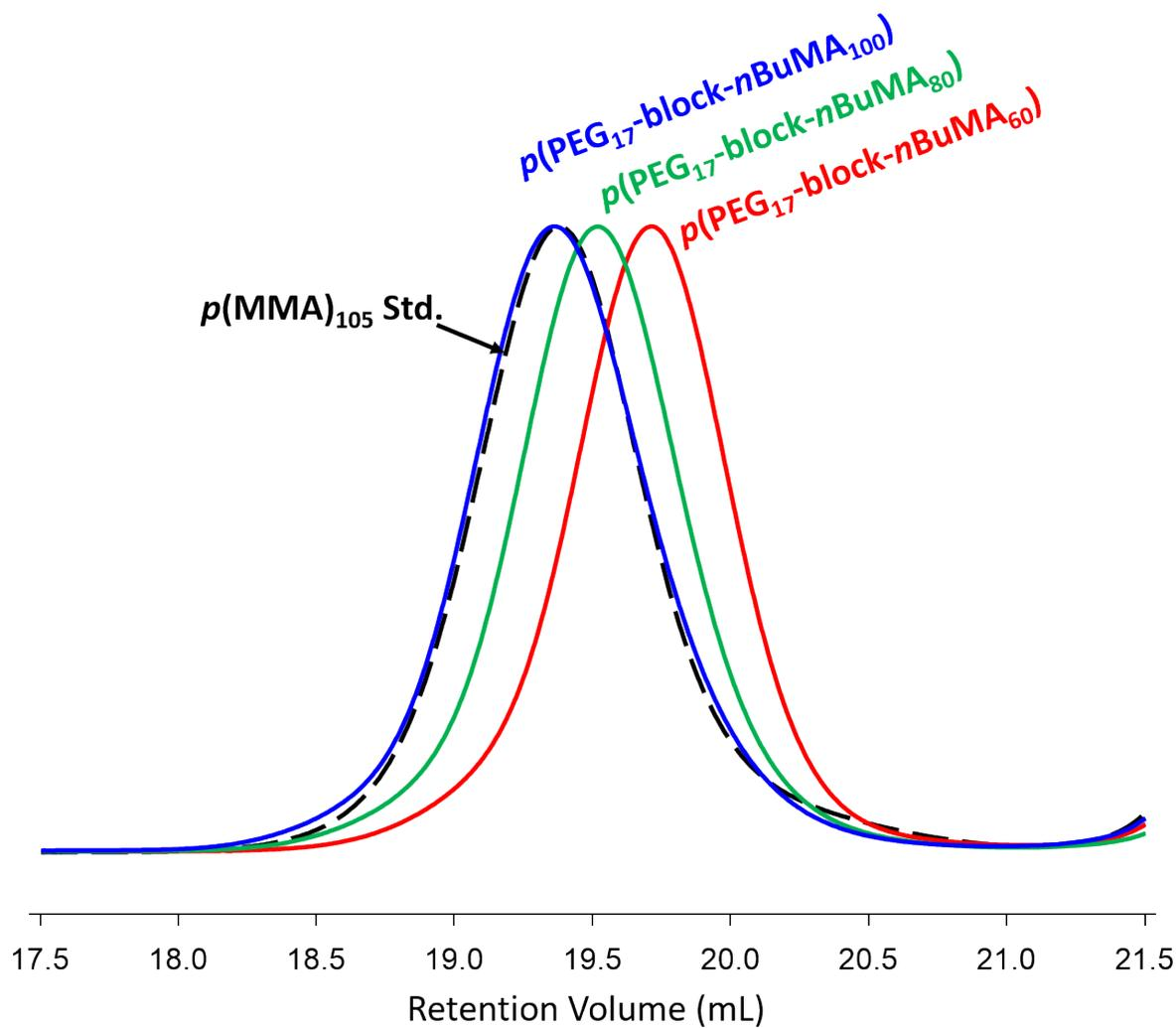
**Figure S10** Overlaid SEC chromatograms (RI) of  $p(\text{PEG}_{17}\text{-}b\text{-}n\text{BuMA}_x)$  A-B block copolymers produced *via* methanolic Cu-catalysed ATRP of  $n\text{BuMA}$  at 60 °C using  $\text{PEG}_{17}\text{-Br}$  macroinitiator across the targeted  $\text{DP}_n = 60\text{-}100$  monomer units -  $p(\text{MMA})_{105}$  standard (black dotted trace) shown for comparison. Analysis performed by triple detection SEC with a mobile phase of DMF (+ 0.01M LiBr) at 1 mL/min, 60 °C.
