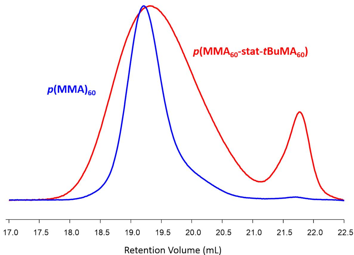
**Figure S24** SEC chromatogram (RI) of the  $p(\text{MMA}_{60}\text{-stat-}t\text{BuMA}_{60})$  statistical copolymer produced *via* methanolic Cu-catalysed ATRP of MMA and *t*BuMA at 60 °C, targeting  $\text{DP}_n = 60$  monomer units for each comonomer –  $p(\text{MMA})_{60}$  homopolymer (blue trace) overlaid for comparison. Analysis performed by triple detection SEC with a mobile phase of THF (+ 2 v/v % TEA) at 1 mL/min, 35 °C.
