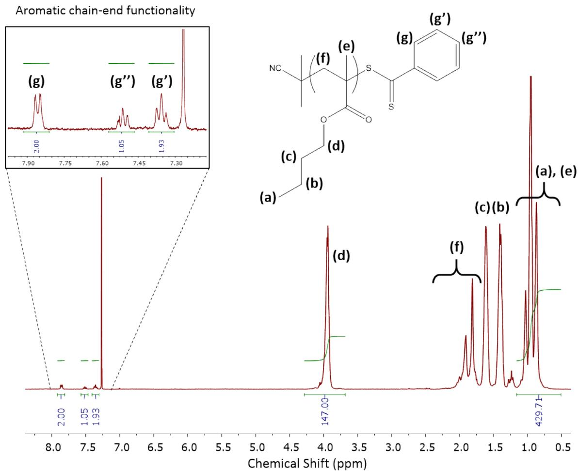
**Figure S1**  $^1\text{H-NMR}$  ( $\text{CDCl}_3$ ) analysis of purified  $p(n\text{BuMA})_{60}$  obtained *via* RAFT to determine the DPn. Inset: magnification of the aromatic region of the spectrum showing resonances attributed to the CTA Z-group chain-end functionality.
