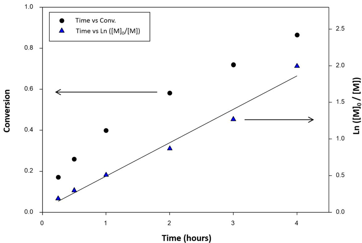
**Figure S14;** Kinetic studies of  $p(\text{PEG}_{45}\text{-}b\text{-}n\text{BuMA}_{80})$  synthesis *via* Cu-Catalysed ATRP in anhydrous methanol at 60 °C showing conversion and semilogarithmic plots *vs.* time.
