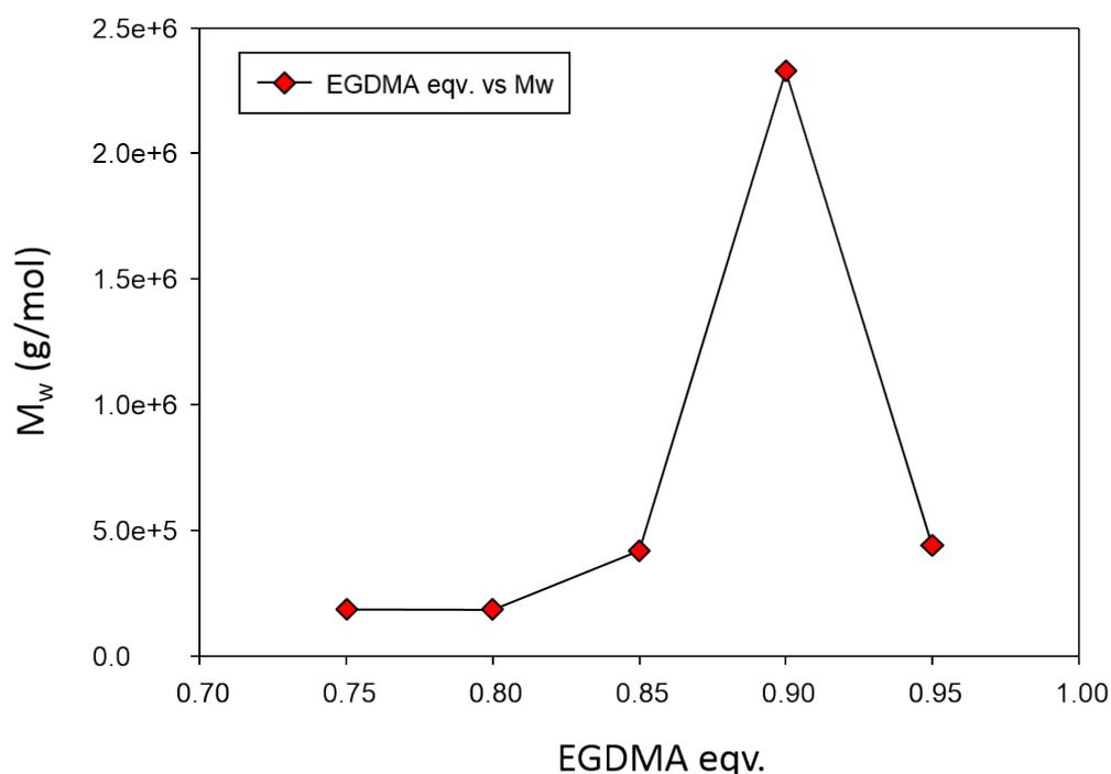
**Figure S19** Evolution of the weight average molecular weight ( $M_w$ ) with increasing levels of divinyl monomer, EGDMA (0.75 to 0.95 molar equivalent wrt. macroinitiator), for the Cu-catalysed branched methanolic ATRP of *n*BuMA (targeted  $DP_n = 60$  monomer units per primary chain) at 60 °C using PEG<sub>113</sub>-Br macroinitiator. The observed decrease in  $M_w$  at 0.95 equivalent EGDMA indicates onset of microgel formation.
