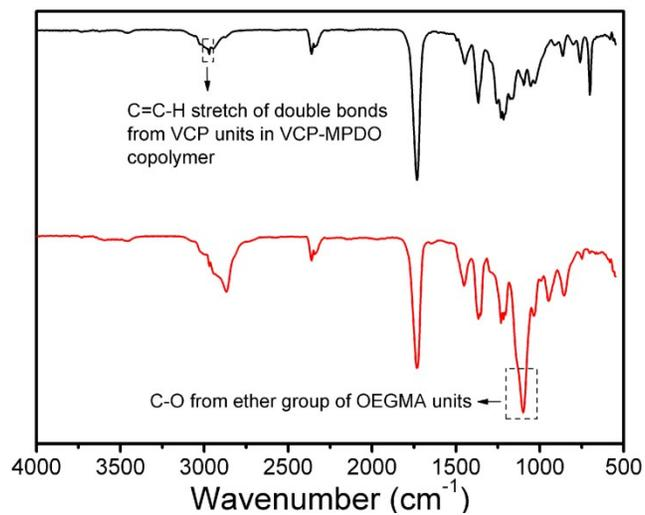
**Figure S2.** IR spectra of original VCP-MPDO copolymers (black) and APCNs (gel-3) after purification (red).
