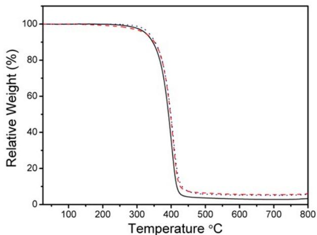
**Figure S5.** TGA profiles of VCP-MPDO copolymers with different comonomer ratios in feed.
