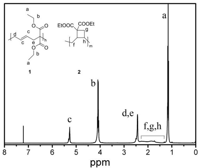
**Figure S1.** <sup>1</sup>H-NMR spectrum of VCP homopolymer prepared at 120 °C. Structure 1: VCP unit with ring-opened structure in PVCP; structure 2: VCP unit with ring-closed structure in PVCP.
