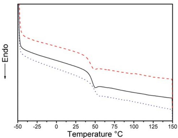
**Figure S6.** DSC heating traces of VCP-MPDO copolymers with different comonomer ratios in
