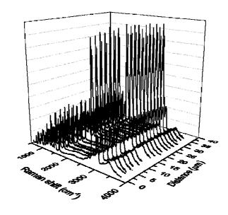
**Figure S1.**Confocal-Raman spectra along the cross-section of (A) **PTDAMPB** and (b) **PVBTAC** pore-filling membranes in the region of 500 cm<sup>-1</sup>to 3500 cm<sup>-2</sup> confirming pore-filling by the polyelectrolytes.
