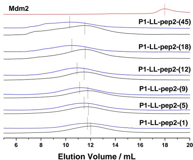
**Figure S9.** Gel filtration chromatograms show the elution of **P1-LL-pep2-(n)** (n = 1, 5, 9, 12, 18 and 45) before (black line) and after (blue line) incubation with Mdm2 (molar feed ratio of **pep1**/Mdm2 = 1:1) on Superdex-200 column. Samples were eluted by 1×PBS, pH 7.4, at a rate of 0.45 mL/min at 4 °C.
