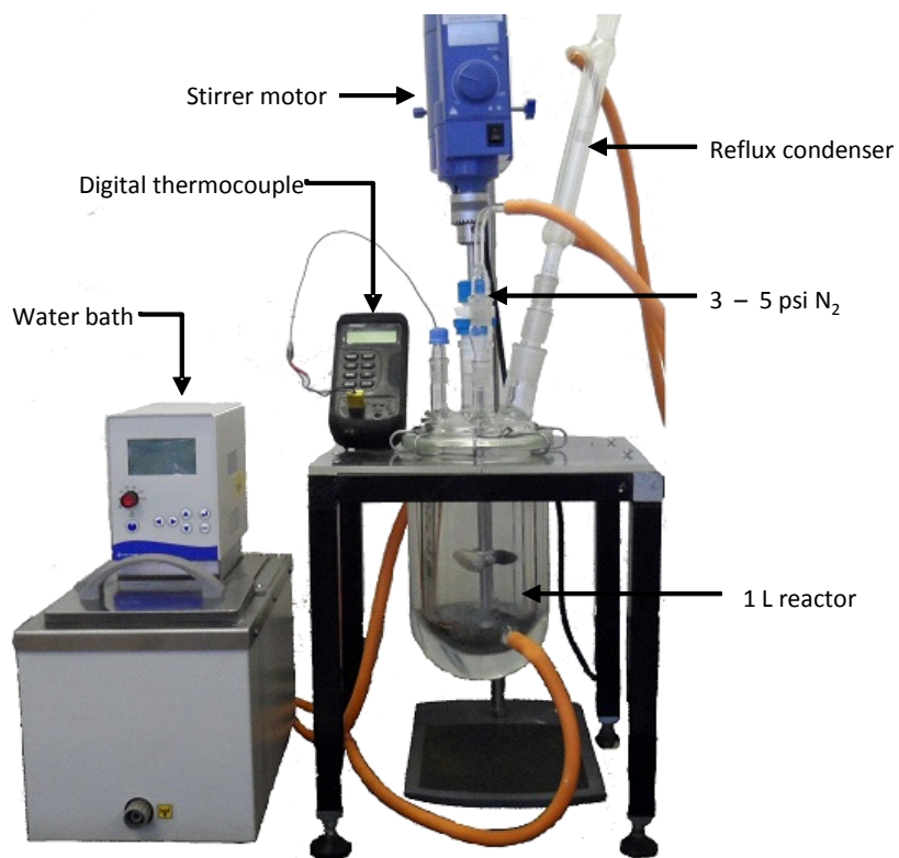
Experimental set-up for suspension polymerisation
