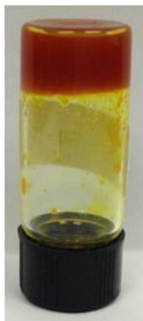
Figure S15. Picture for the organogel fabricated from 1 and TBACl (1:3) in \text{CHCl}_3 .
