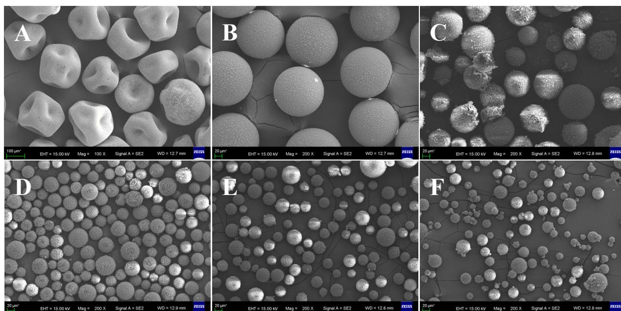
**Figure S4** SEM images of GMA loaded microcapsules made with different hydrolyzed PGMA particle concentration: (A) 0.5% (B) 1%, (C) 2%, (D) 3%, (E) 4%, (F) 5%. All microcapsules were
