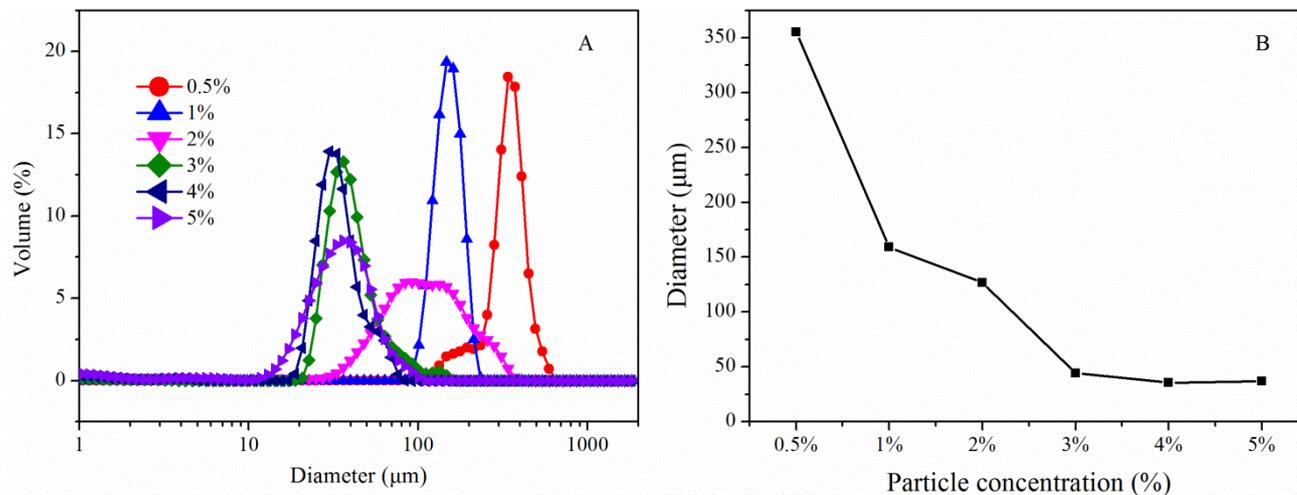
**Figure S5** The size distributions of GMA loaded microcapsules prepared under various hydrolyzed PGMA particle concentration and (B) Diameters as a function of particle concentration. All microcapsules were made with 70% designed weight ratio of GMA in the mixed oil phase.
