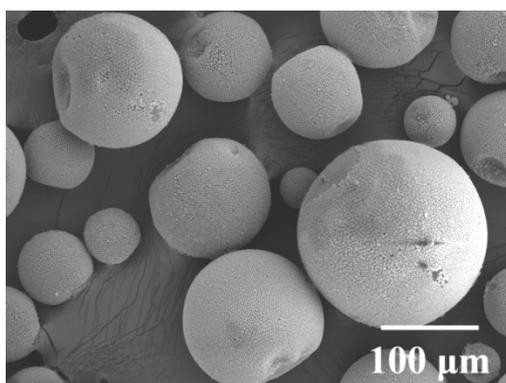
**Figure S2** SEM image of the shell materials obtained in the same condition as the microcapsules (sample 3) except that the TTT was not added.
