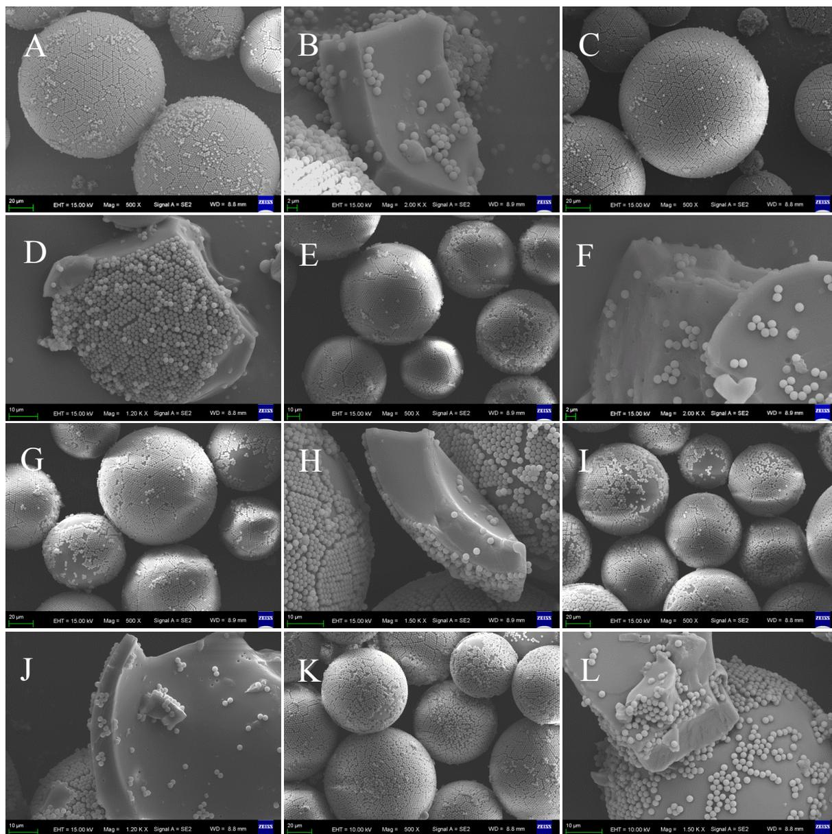
**Figure S6** SEM images of integrated and ruptured TTT loaded microcapsules under different stirring speeds: (A), (B) 500 rpm; (C), (D) 800 rpm; (E), (F) 1000 rpm; (G), (H) 1200 rpm; (I), (J) 1500 rpm; (K), (L) 1800 rpm. The microcapsules were made as the same recipe of sample 3 except that the emulsification method was stirring instead of shaking by hand.
