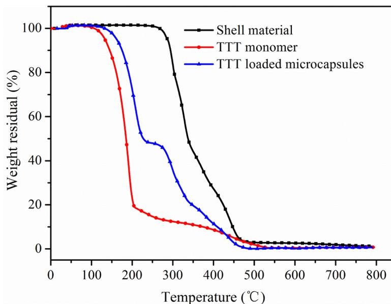
**Figure S3** TGA curves: shell material■, TTT monomer● and TTT loaded microcapsules▲. The microcapsules were sample 3. The shell material was obtained in the same condition as sample 3 except that the TTT was not added and its SEM image is given in Figure S3. TGA measurements were performed under the condition that temperature was raised from 25 to 800 °C.
