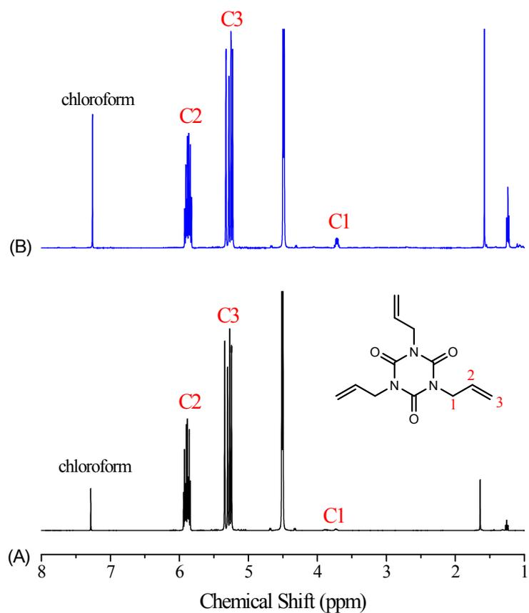
**Figure S1** <sup>1</sup>H NMR spectra of (A) TTT monomer and (B) the extracted core of TTT loaded microcapsules (sample 3) in chloroform-d.
