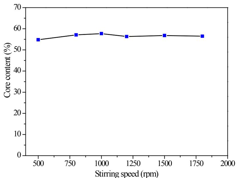
**Figure S7** The core content of TTT loaded microcapsules as a function of stirring speed. The microcapsules were made as the same recipe of sample 3 except that the emulsification method was stirring instead of shaking by hand.
