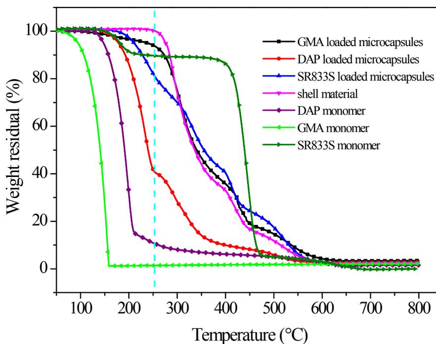
**Figure S10** the TGA curves of different core monomers and microcapsules.
