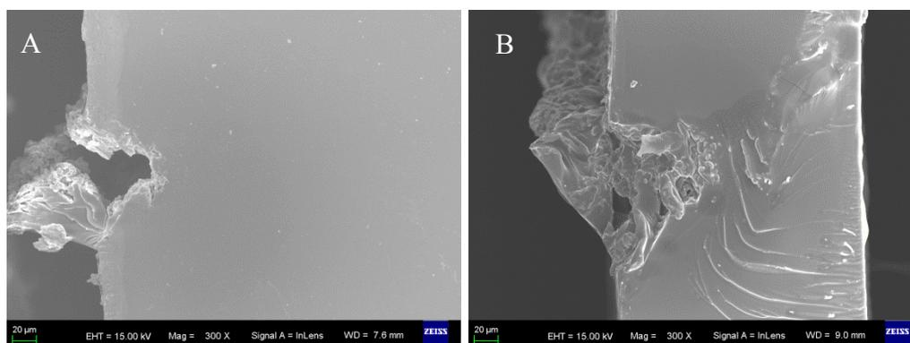
**Figure S9** SEM images of the cross section of TTT loaded microcapsules (sample 6) embedded in cured epoxy coatings with scratched cracks: (A) without any treatment and (B) cracks irradiated under UV for 10 min after injecting the mixture of TMMP and photoinitiator 184.
