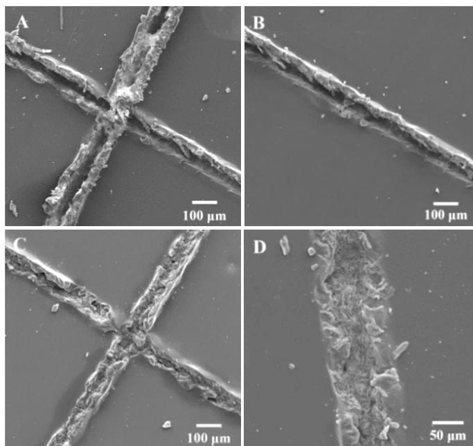
**Figure S8** SEM images of TTT loaded microcapsules (sample 6) embedded in cured epoxy coatings with scratched cracks: (A) without any treatment, (B) cracks irradiated under UV for 10 min, (C) cracks irradiated under UV for 10 min after injecting the mixture of TMMP and photoinitiator 184
