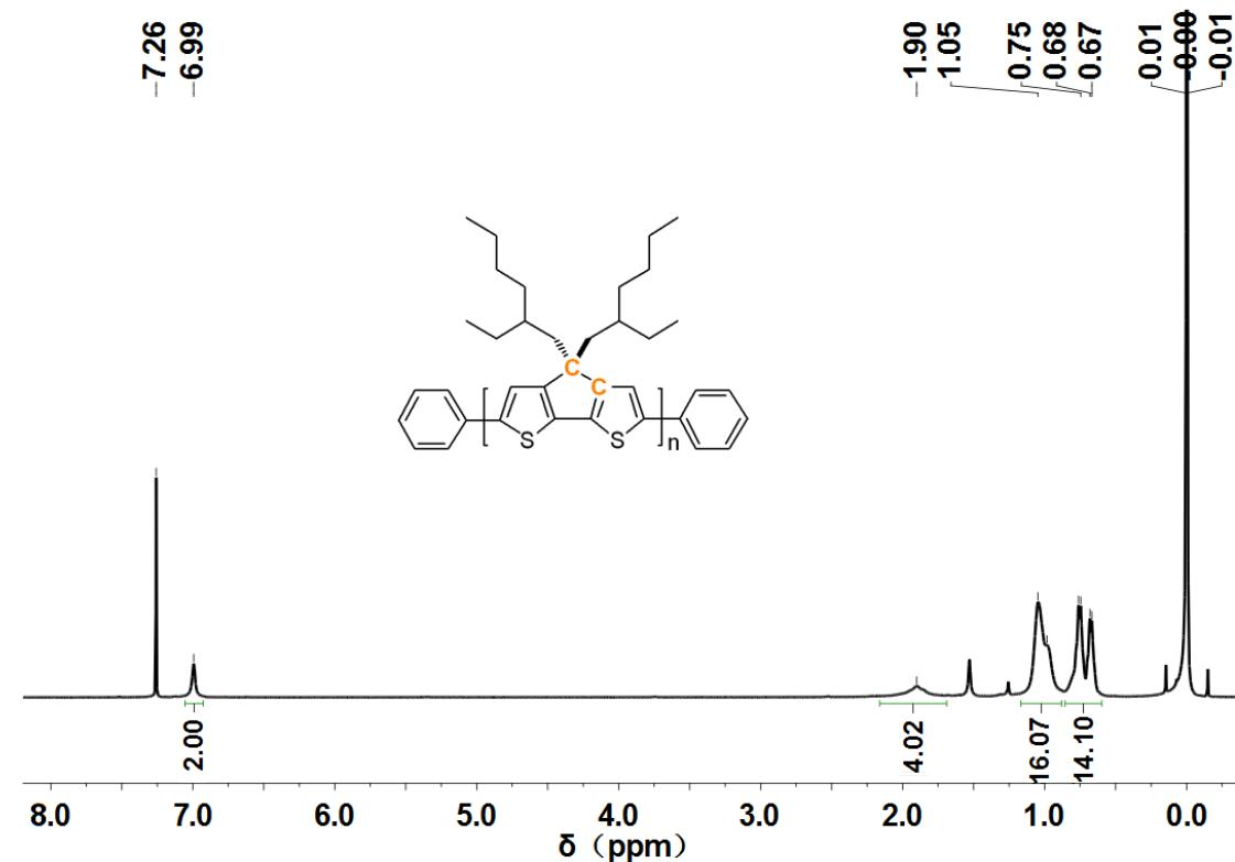
Figure S2.  $^1\text{H}$  NMR spectrum of polymer PCPDT in  $\text{CDCl}_3$  at 25 °C.
