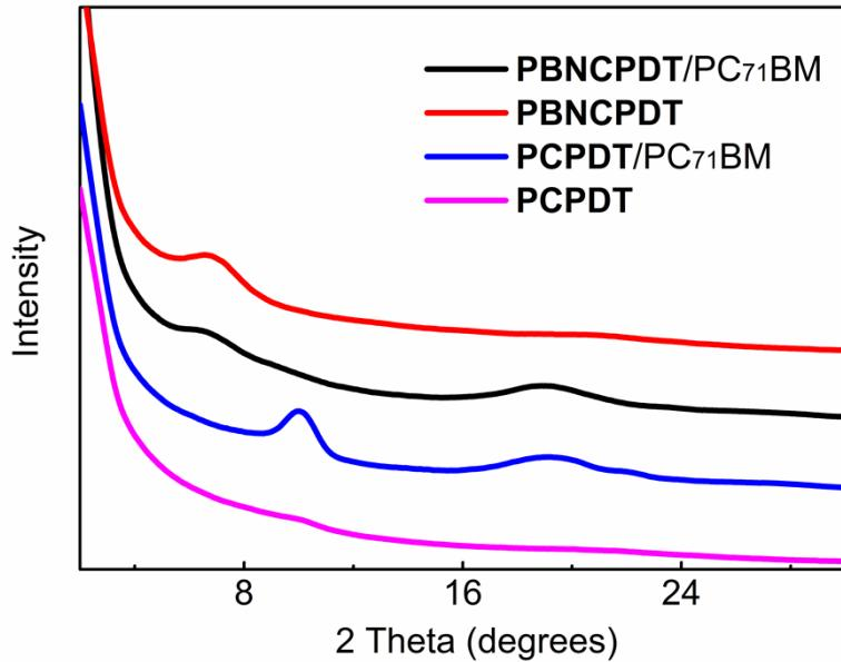
**Figure S6.** Out-of plane grazing incidence X-ray diffraction (GI-XRD) patterns of the prime films and blend films from *o*-DCB/DIO solutions. Compared with the **PCPDT** prime films, **PBNCPDT** shows much more ordered and crystalline packing structures with diffraction peak around 6.7 °. In the blend films, both of them show improved ordered structures.
