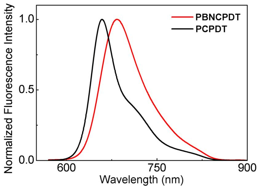
**Figure S4.** Normalized fluorescence spectra of **PBNCPDT** and **PCPDT** in *o*-DCB ( $\lambda_{\text{ex}} = 570$  nm).
