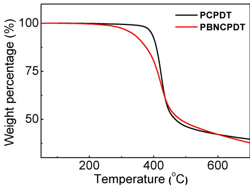
**Figure S3.** TGA curves of PBNCPDT and PCPDT.
