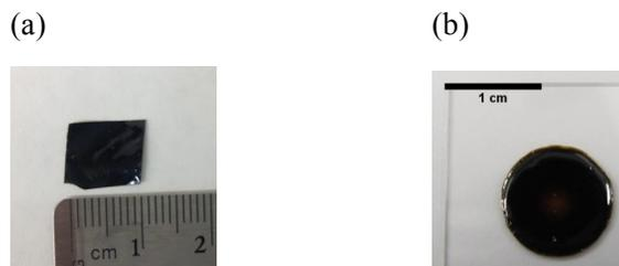
**Figure S7.** (a) Free-standing film of phmTTFMA; (b) phmTTFMA-chloranil film on glass substrate for electrical conductivity measurement.
