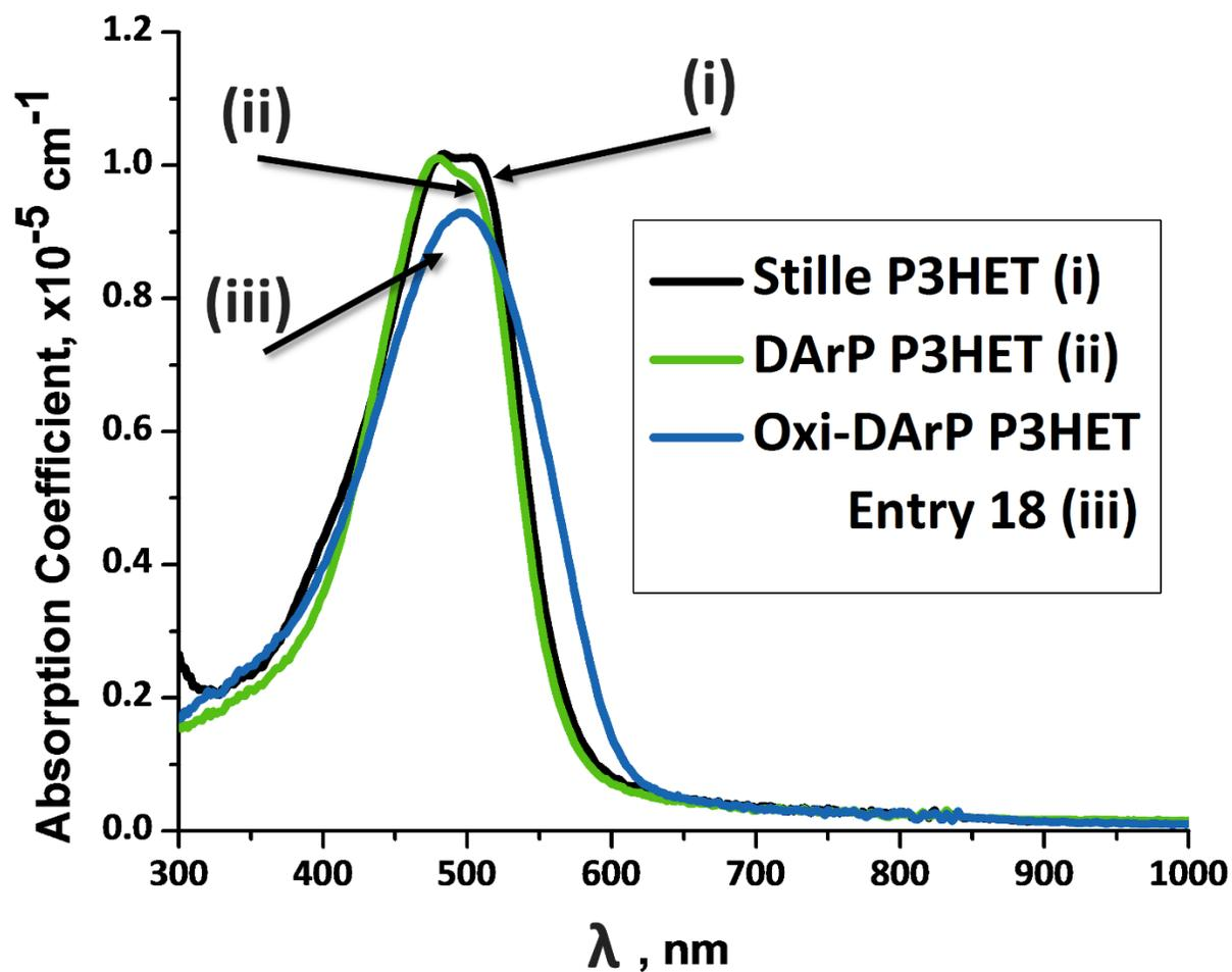
**Figure S31.** Comparison of the UV-Vis Spectra for **Stille P3HET (i)**, **DArP P3HET (ii)**, and **Oxi-DArP P3HET Entry 18 (iii)**.
