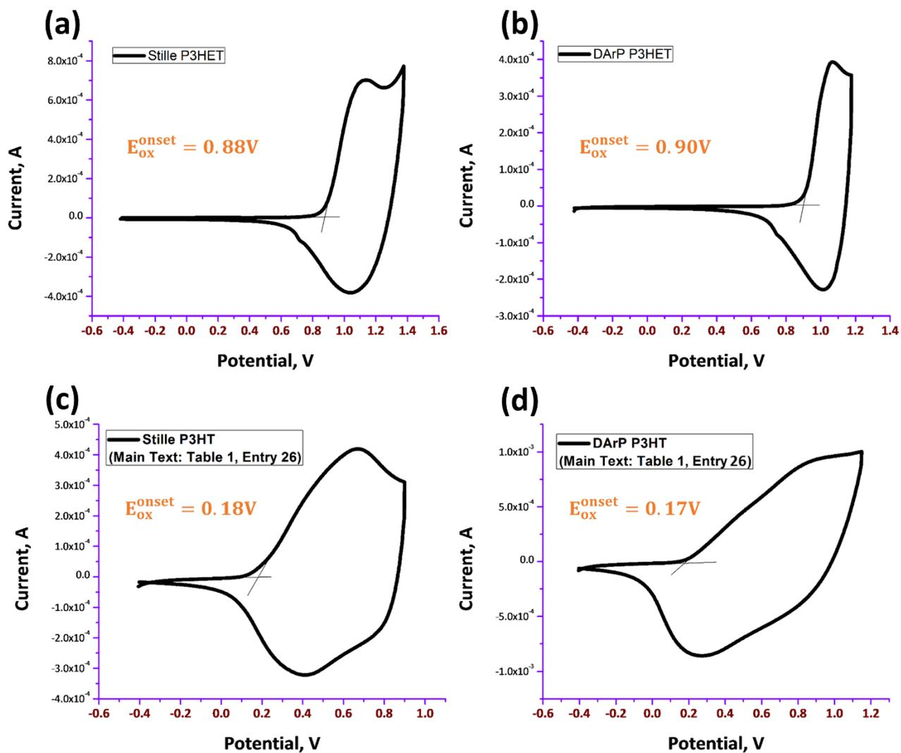
**Figure S25.** CV Traces for the electrochemical oxidation of Stille P3HET (a), DArP P3HET (b), Stille P3HT (c), and DArP P3HT (d).
