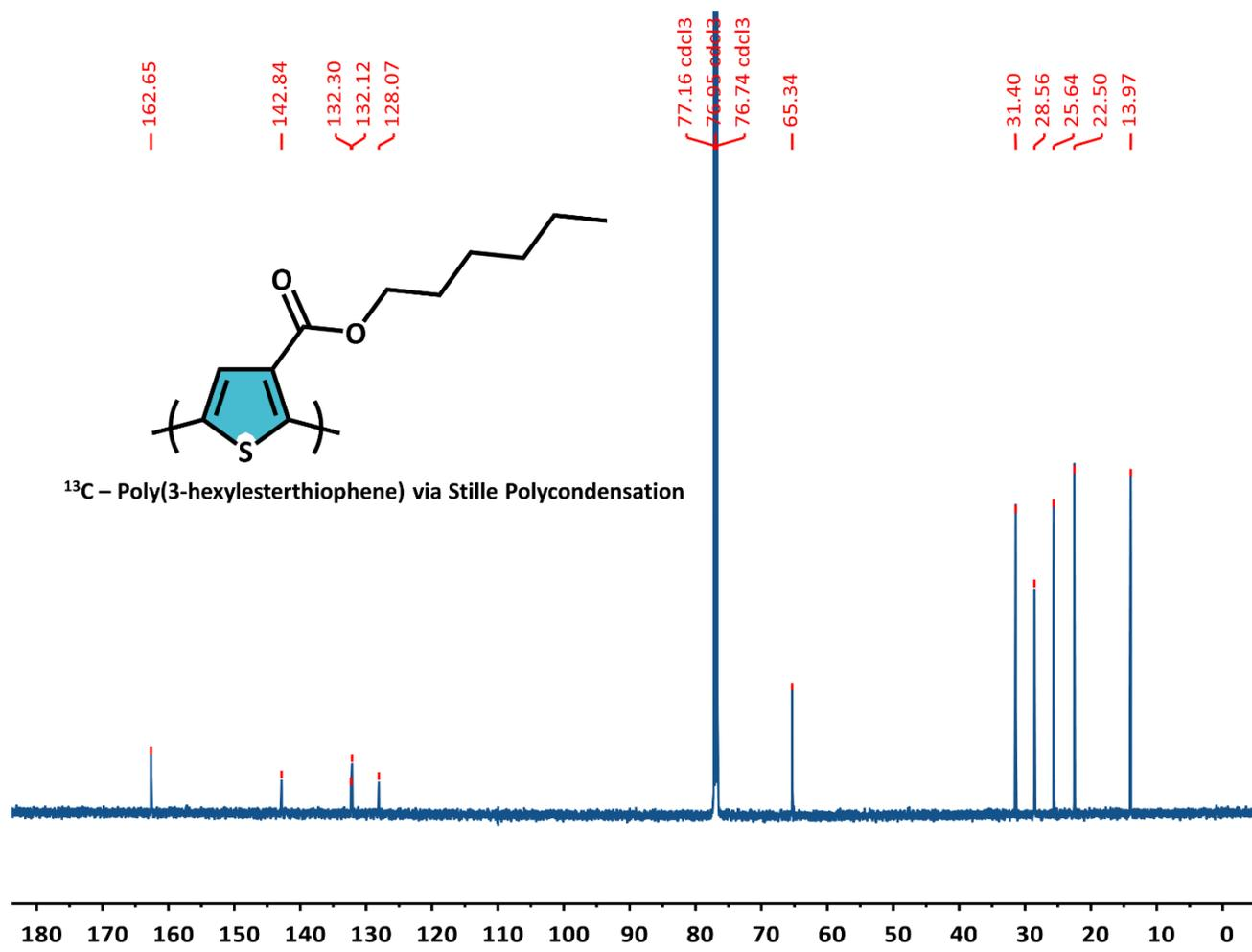
Figure S22. <sup>13</sup>C-NMR of Stille P3HET in CDCl<sub>3</sub>.
