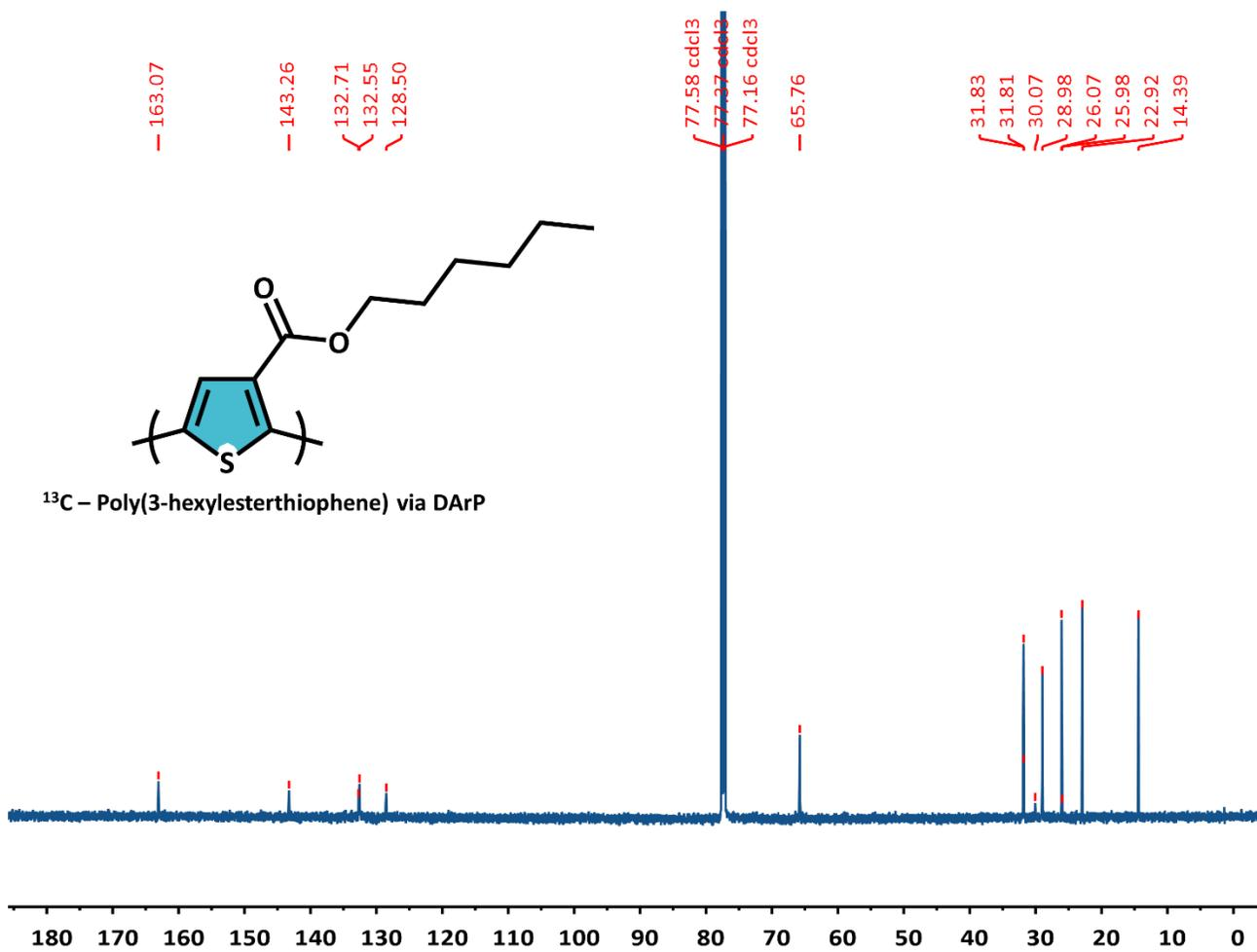
Figure S23. <sup>13</sup>C-NMR of DArP P3HET in CDCl<sub>3</sub>.
