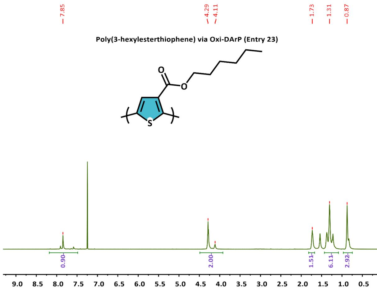
**Figure S20.** <sup>1</sup>H-NMR of Oxi-DArP P3HET (Entry 23) in CDCl<sub>3</sub>.
