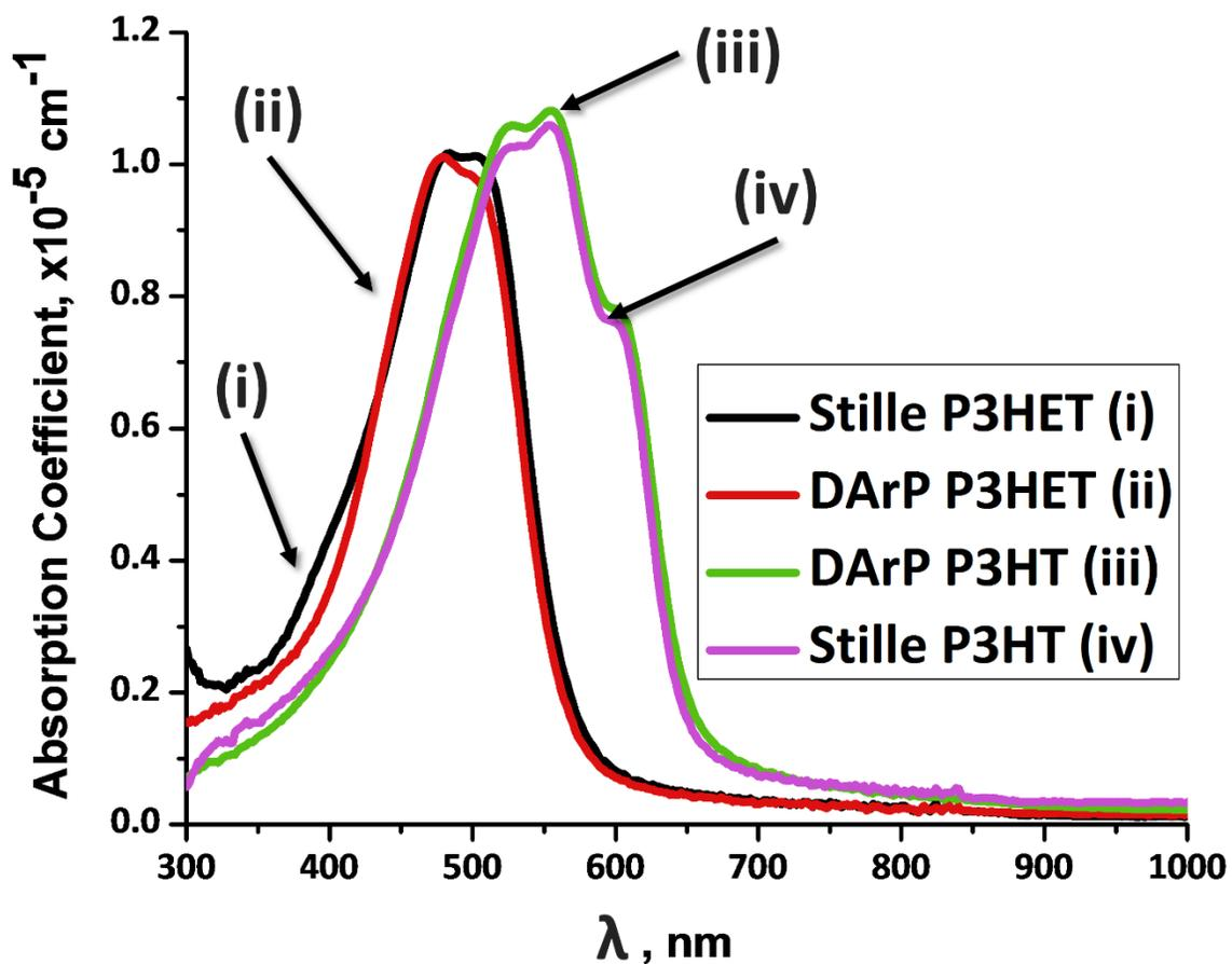
Figure S28. UV-Vis Spectra for Stille P3HET (i), DArP P3HET (ii), DArP P3HT (iii), and Stille P3HT (iv).
