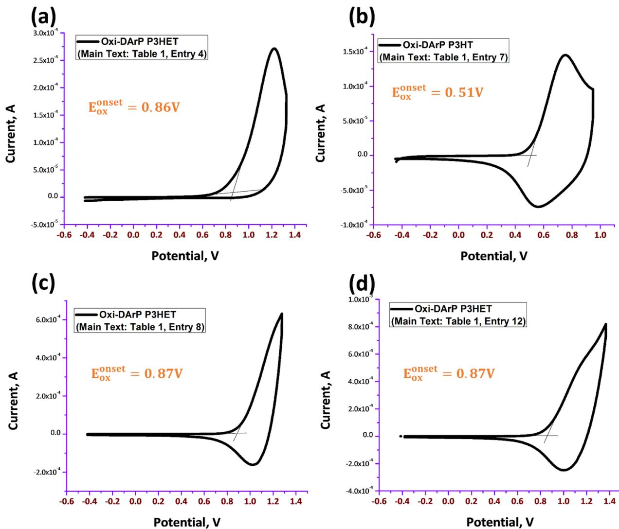
Figure S26. CV Traces for the electrochemical oxidation of **Entry 4** (a), **Entry 7** (b), **Entry 8** (c), and **Entry 12** (d).
