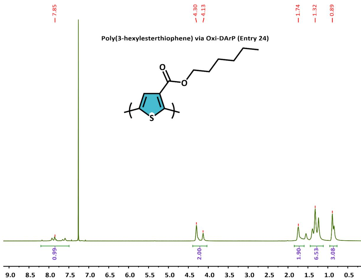
Figure S21. <sup>1</sup>H-NMR of Oxi-DArP P3HET (Entry 24) in CDCl<sub>3</sub>.
