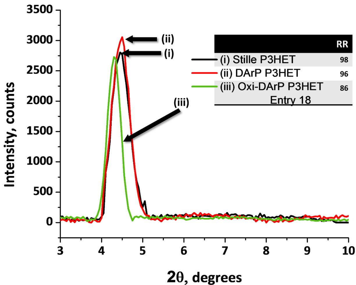
Figure S34. Comparison of GIXRD Spectra for **Stille P3HET** (i), **DArP P3HET** (ii), and optimized **Oxi-DArP P3HET Entry 18** (iii). The regioregularity of the corresponding polymers is provided as well.
