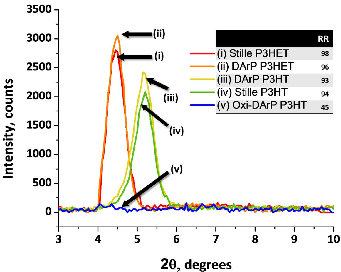
**Figure S32.** GIXRD Spectra for **Stille P3HET (i)**, **DArP P3HET (ii)**, **DArP P3HT (iii)**, **Stille P3HT (iv)**, and **Oxi-DArP P3HT Entry 7 (v)**. The regioregularity of the corresponding polymers is provided as well.
