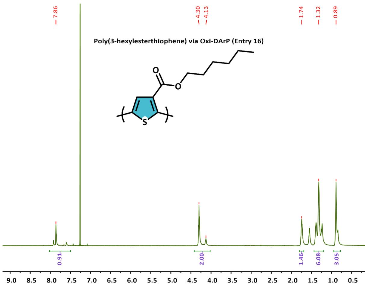
Figure S17. <sup>1</sup>H-NMR of Oxi-DArP P3HET (Entry 16) in CDCl<sub>3</sub>.
