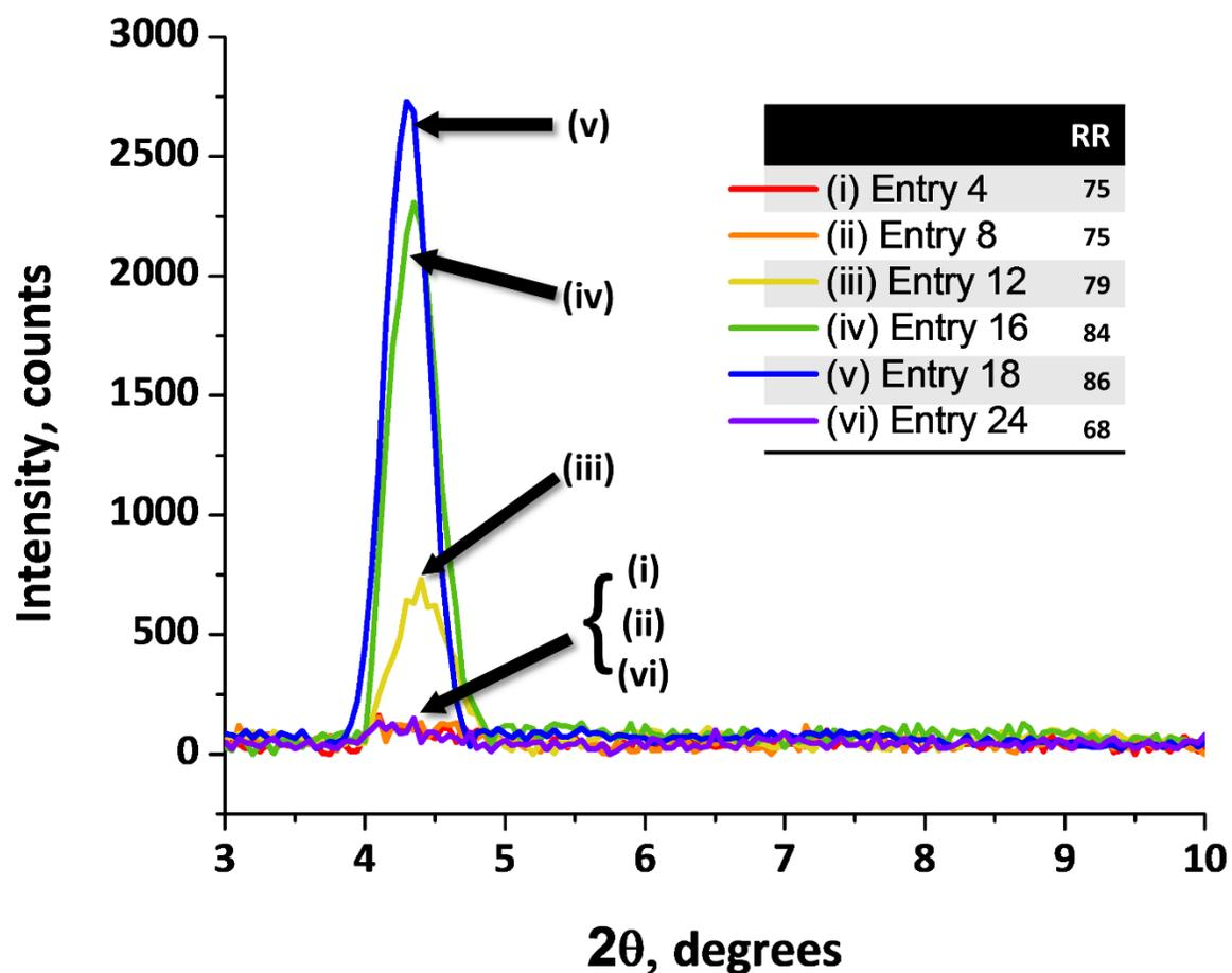
**Figure S33.** GIXRD Spectra for Oxi-DArP P3HET Entry 4 (i), Oxi-DArP P3HET Entry 8 (ii), Oxi-DArP P3HET Entry 12 (iii), and Oxi-DArP P3HET Entry 16 (iv), Oxi-DArP P3HET Entry 18 (v), Oxi-DArP P3HET Entry 24 (vi). The regioregularity of the corresponding polymers is provided as well.
