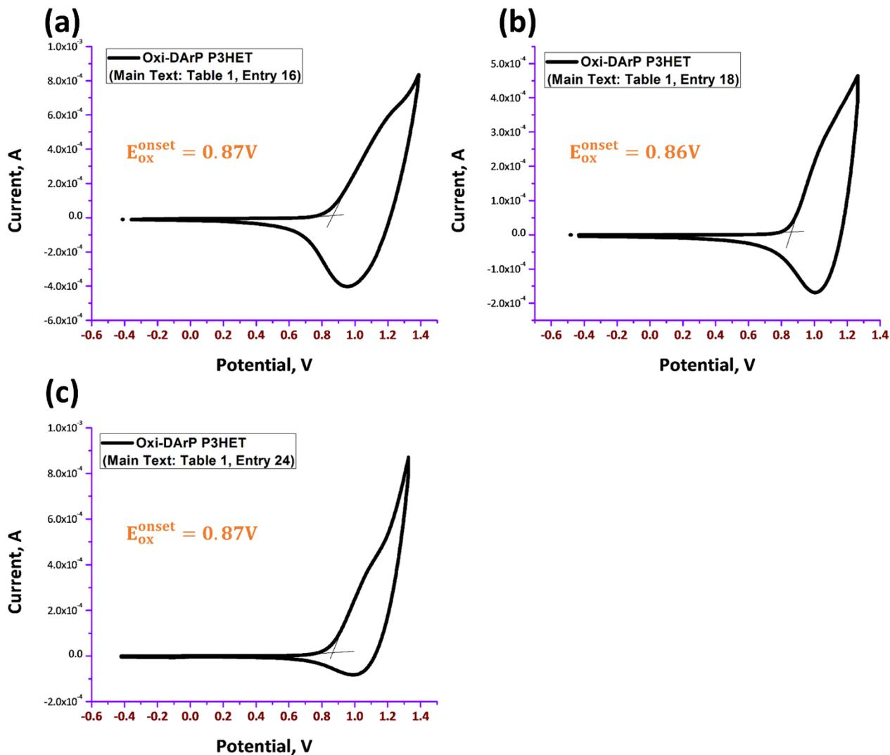
Figure S27. CV Traces for the electrochemical oxidation of Entry 16 (a), Entry 18 (b), Entry 24 (c).
