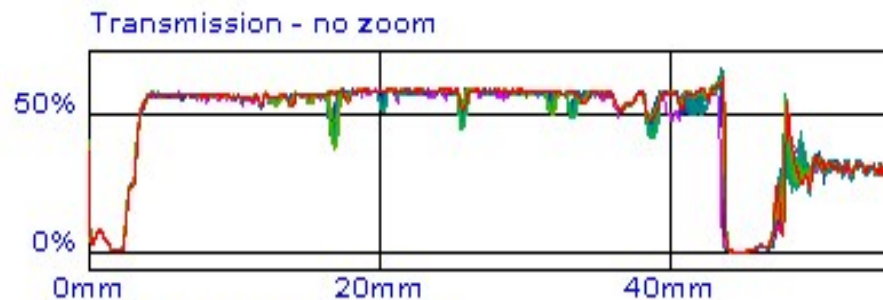
Fig. S4 Stability of the diluted dispersion of silica obtained through light scattering by use of TURBISCAN LAB expert , during 10 hours at ambient temperature.
