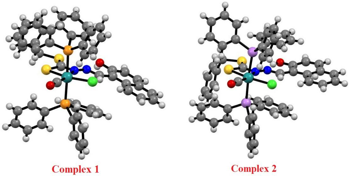
**Fig. S8** LANL2DZ and 6-31G\* (d, p) ground state optimized geometry of complexes **1, 2**
