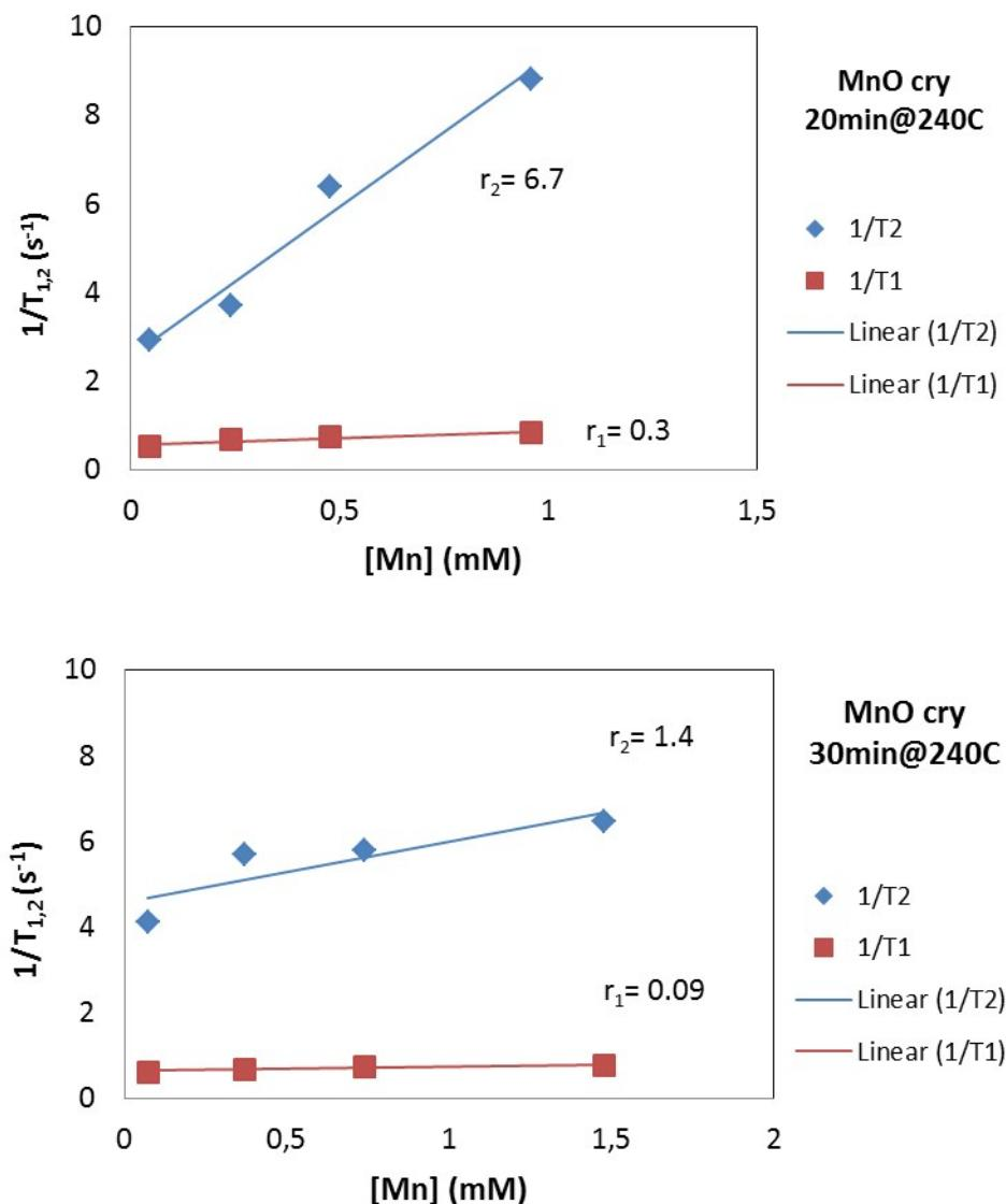
**Supplementary Figure 1.** Relaxivity plots for the as-prepared crystalline samples MnO 20min@240C and 30min@240C in water as measured on a minispec mq60 NMR spectrometer.
