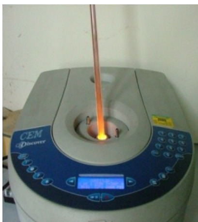
Fig. S1 Photograph showing a reaction in progress demonstrating the occurrence of an orange-yellow glow following Li evaporation.
