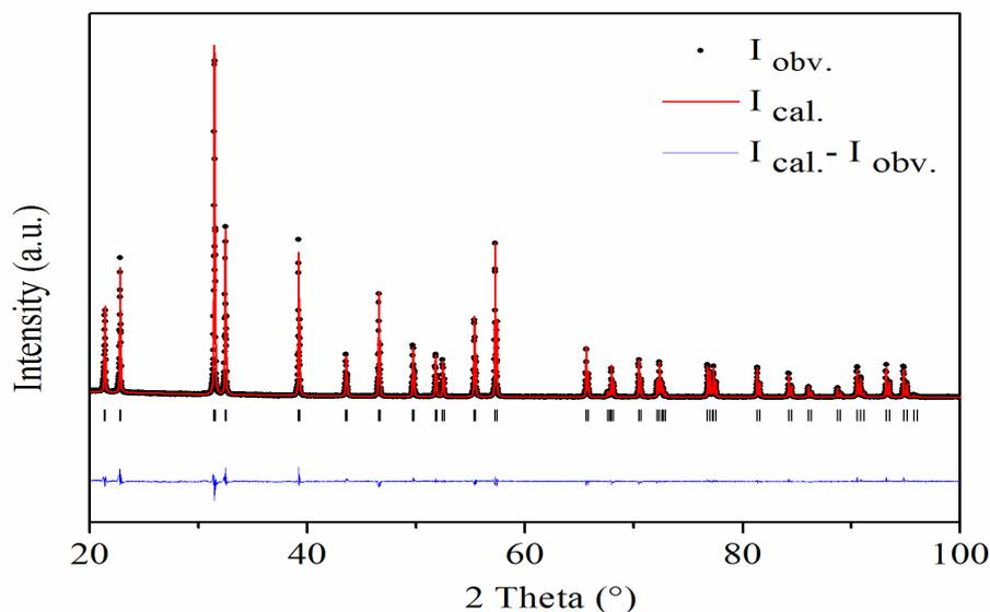
Fig. S3 Observed (point), calculated (line) and difference profiles at room temperature after Rietveld refinement using  $P4mm$  space group for PT
