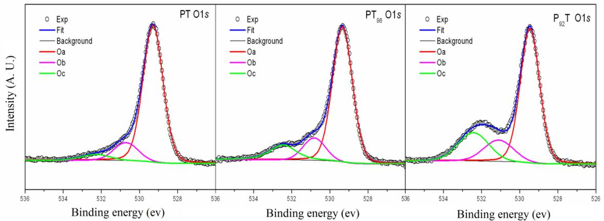
**Fig. S5.** O 1s XPS spectra of PT, PT<sub>98</sub> and P<sub>92</sub>T with peak fitting
