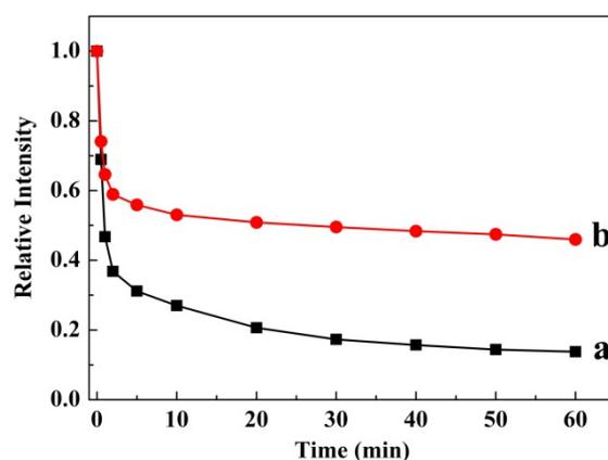
**Fig. S12** The fluorescence quenching curves for P2 (100 nM)/MOF (20 μg/mL) composite as a function of time (a) in the absence of Hg<sup>2+</sup> and (b) in the presence of Hg<sup>2+</sup> of 10 μM. The excitation and emission wavelengths are 480 and 517 nm.
