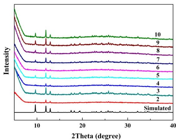
**Fig. S6** Power X-ray diffraction pattern of compound GdL after being immersed in the solution of pH = 2-10 for two weeks.
