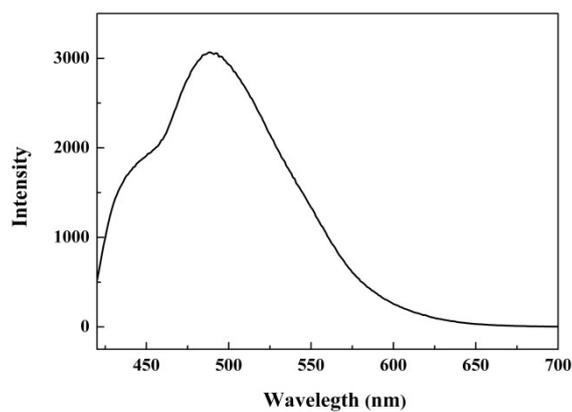
**Fig. S8** Room-temperature emission spectra for GdL in the solid state excited at 405
