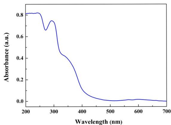
**Fig. S7** The UV-Vis diffuse reflectance spectra (DRS) of GdL.
