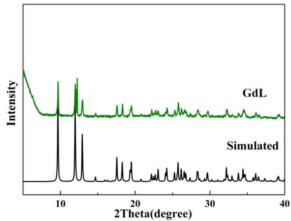
**Fig. S3** Power X-ray diffraction pattern of simulated and experimental as-synthesized compound GdL.
