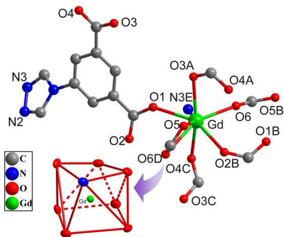
**Fig. S1** Local coordination environment of the GdIII ions in GdL. Hydrogenatoms attached to carbon atoms are omitted for clarity. Symmetry codes: A: $-x, -y, -z$ ; B: $0.5-x, 0.5+y, 0.5-z$ ; C: $0.5+x, -0.5-y, 0.5+z$ ; D: $0.5-x, -0.5+y, 0.5-z$ ; E: $1-x, -1-y, -z$ .
