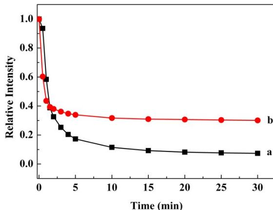
**Fig. S10** The fluorescence quenching curves for P1 (50 nM)/MOF (5  $\mu\text{g/mL}$ ) composite as a function of time (a) in the absence of T1 and (b) in the presence of T1 of 50 nM. The excitation and emission wavelengths are 494 and 517 nm.
