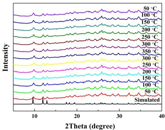
**Fig. S5** Power X-ray diffraction pattern of simulated and experimental as-synthesized compound GdL from 50 °C to 350 °C, then from 350 °C to 50 °C.
