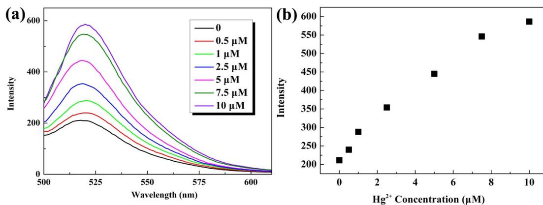
**Fig. S14** (a) Fluorescence spectra of P2/GdL in the presence of different concentrations of  $\text{Hg}^{2+}$  in Tris-HCl buffer (pH = 7.4) (from bottom to top: 0, 0.5, 1, 2.5, 5, 7.5, and 10  $\mu\text{M}$ ). Excitation was at 480 nm and emission intensity was recorded at 517 nm; (b) the corresponding fluorescence intensity plotted against  $\text{Hg}^{2+}$  concentration.
