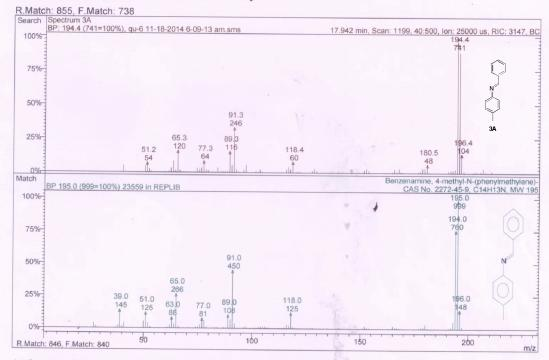
1st Spectrum from ...ws\data\2014\nov\qu-6 11-18-2014 6-09-13 am.sms Scan No: 1199, Time: 17.942 minutes No averaging. Background corrected. Comment: 17.942 min. Scan: 1199 40:500 Ion: 25000 us RIC: 4272 Pair Count: 98 MW: 0 Formula: None CAS No: None Acquired Range: 39.5 - 500.5 m/z
