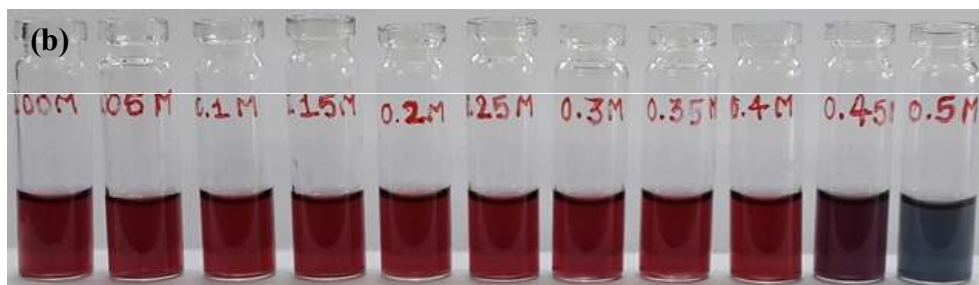
Figure S7. (a) UV-visible absorption spectra of PCA-DTC-Au NPs in the presence of different concentrations of NaCl (0.05 to 0.50 M). (b) photographic image of PCA-DTC-Au NPs after addition of different concentrations of NaCl (0.05 to 0.50 M).
