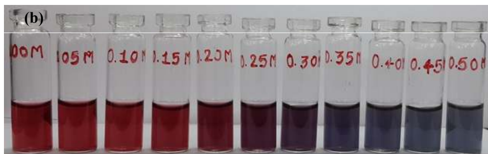
Figure S8. (a) UV-visible absorption spectra of PCA-DTC-Au NPs in the presence of different concentrations of NaCl (0.05 to 0.50 M) along with 100 \mu\text{M} of \text{Al}^{3+} ion. (b) photographic image of PCA-DTC-Au NPs after addition of different concentrations of NaCl (0.05 to 0.50 M) along with 100 \mu\text{M} of \text{Al}^{3+} ion.
