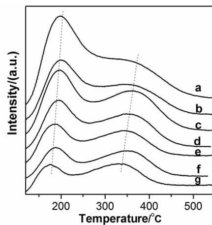
**Fig. S1** NH<sub>3</sub>-TPD profiles of the parent and oxalic acid-treated H-MCM-22 samples; (a) H-MCM-22-15, (b) H-MCM-22-15-o, (c) H-MCM-22-25, (d) H-MCM-22-25-o, (e) H-MCM-22-37, (f) H-MCM-22-37-o and (g) H-MCM-22-50.
