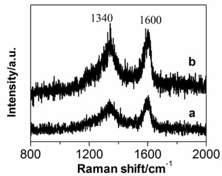
**Fig. S7** Raman spectra of the coke species deposited on the (a) H-MCM-22-25 and (b) H-MCM-22-37.
