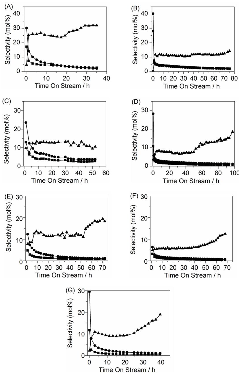
**Fig. S3** Product selectivity obtained over the parent and the oxalic acid-treated H-MCM-22 samples (Reaction conditions: 450 °C, WHSV of 2 h<sup>-1</sup>); (A) H-MCM-22-15; (B) H-MCM-22-15-o; (C) H-MCM-22-25; (D) H-MCM-22-25-o; (E) H-MCM-22-37; (F) H-MCM-22-37-o; (G) H-MCM-22-50; (■) ethane and propane, (●) butane, (▲) C6+ (aliphatic and aromatics hydrocarbons).
