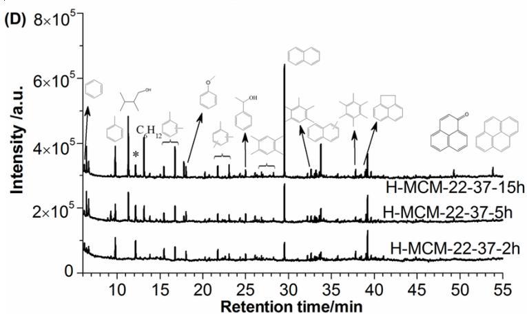
**Fig. S6** GC-MS chromatogram of the coke species extracted with  $\text{CH}_2\text{Cl}_2$  from (A) H-MCM-22-15, (B) H-MCM-22-25, (C) H-MCM-22-25-o and (D) H-MCM-22-37 at different reaction time (Reaction conditions: 450 °C, WHSV = 2 h<sup>-1</sup>. The asterisk (\*) represents the internal standard ( $\text{C}_2\text{Cl}_4$ )).
