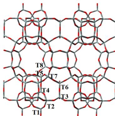
**Scheme S1** MCM-22 framework with 8 crystallographically inequivalent T sites.
