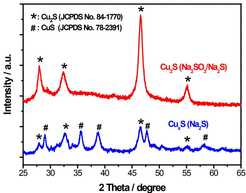
Fig. S2. XRD patterns of  $\text{Cu}_x\text{S} (\text{Na}_2\text{S})$  sample and  $\text{Cu}_2\text{S} (\text{Na}_2\text{SO}_3/\text{Na}_2\text{S})$  sample ( $\text{Cu}_2\text{S}$  achieved by adding  $\text{Cu}^{2+}$  into  $\text{Na}_2\text{SO}_3/\text{Na}_2\text{S}$  solution).
