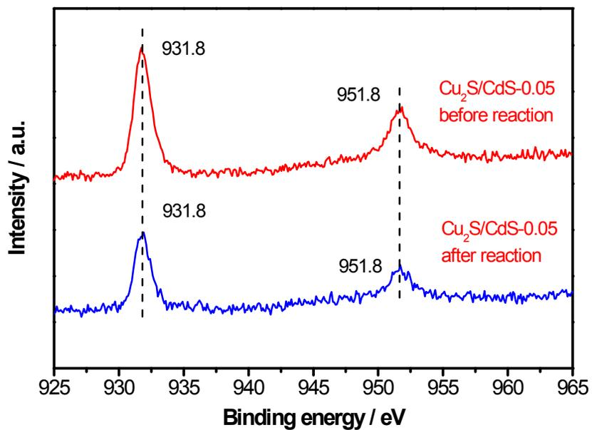
**Fig. S4.** Cu 2p XPS spectra of Cu<sub>2</sub>S/CdS-0.05 sample before and after long-time photocatalytic reaction.
