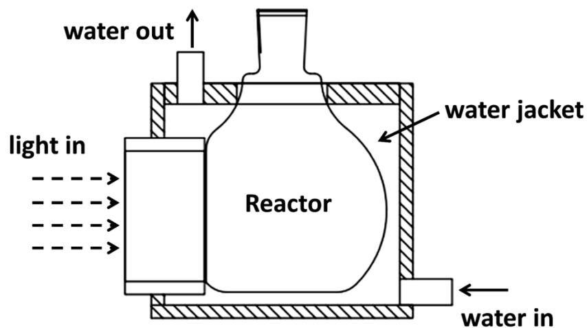
Fig. S1. The schematic diagram of the photocatalytic reactor for hydrogen production.
