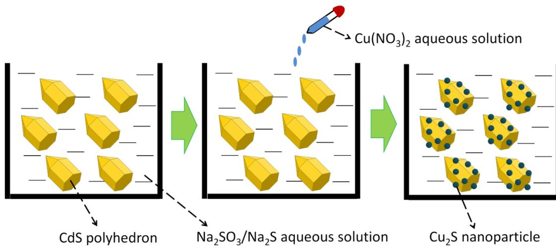
**Fig. S3.** Illustration of the deposition process of Cu<sub>2</sub>S nanoparticles on CdS polyhedrons.
