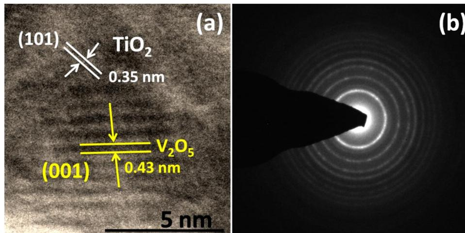
Fig. S3. HRSTEM lattice fringes of  $V_2O_5/TiO_2$  core/shell nanostructures
