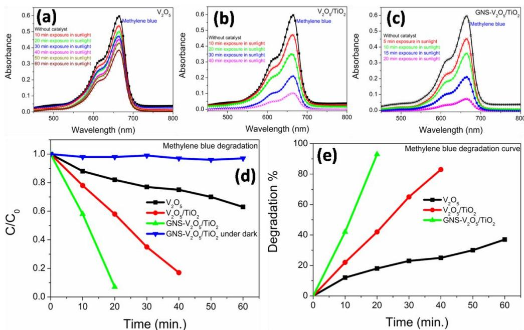
Fig. S1. Photocatalytic degradation of MB using (a)  $V_2O_5$ , (b)  $V_2O_5/TiO_2$ , (c) GNS- $V_2O_5/TiO_2$ , (d) Initial/residual concentration plot vs time and (e) degradation % of MB vs time.
