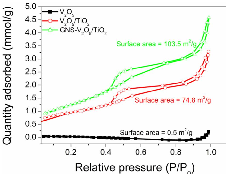
Fig. S2. Nitrogen adsorption – desorption isotherm of  $V_2O_5$ ,  $V_2O_5/TiO_2$  and GNS- $V_2O_5/TiO_2$  nanoarchitecture photocatalysts
