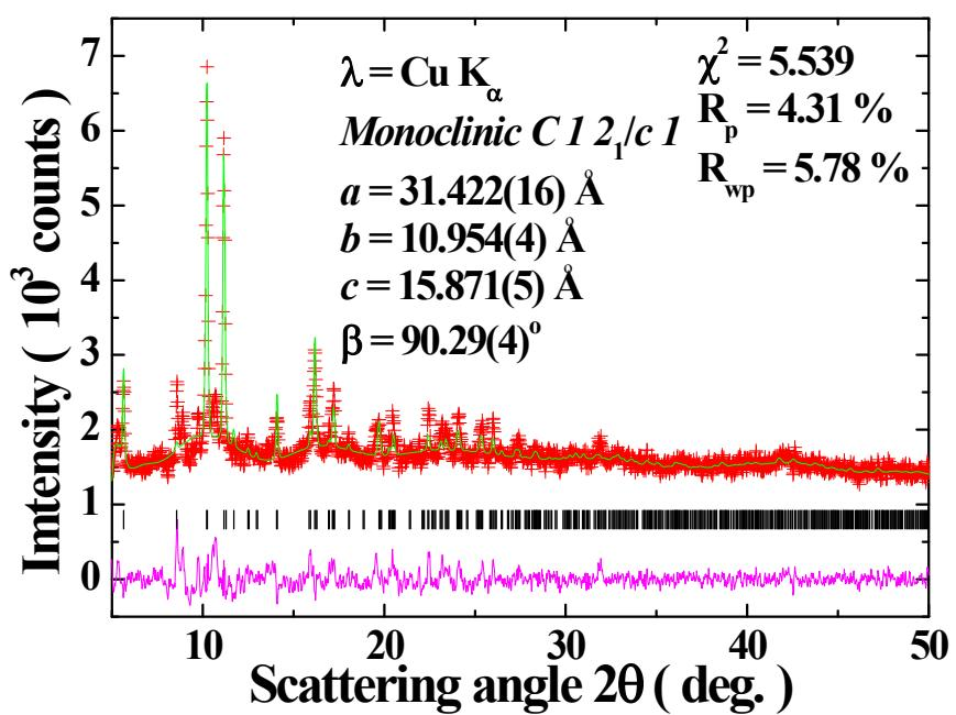
**Fig. S4.** Refinement results of powder X-ray diffraction patterns of **2**, showing observed (red crosses) and calculated (green solid line) spectra and their difference (purple line), with estimated peak positions (black dash).
