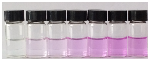
Fig. S8 Color changes of P(HEA-co-RhBBA) in aqueous solution upon addition of varying quantities of \text{Cu}^{2+} ions (from left to right: 0, 0.05, 0.1, 0.25, 0.5, 1.0, 2.0 equiv.).
