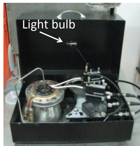
Photo of the black-box chamber for sensing measurement
