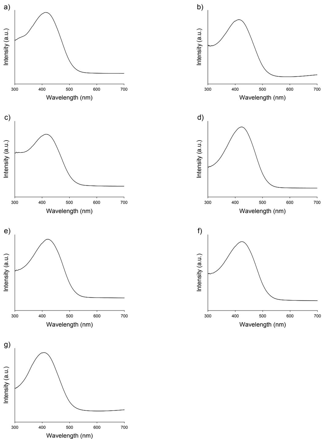
**Figure S2.** UV-vis absorption spectra of P3OT synthesized via FeCl<sub>3</sub>-catalyzed oxidative polymerization with (a) [BmIm][SbF<sub>6</sub>], (b) [BmIm][Tf<sub>2</sub>N], (c) [BmIm][PF<sub>6</sub>], (d) [BmIm][BF<sub>4</sub>], (e) [OmIm][OTf], (f) [BmIm][OTf], and (g) CHCl<sub>3</sub>.
