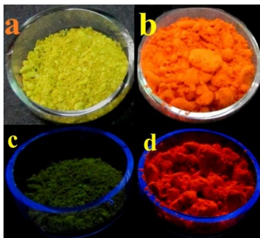
Figure S26 Naked eye colour of AAS (a) and AAS+Zn 2+ adduct (b). (c) and (d) are respective colours under hand held UV lamp.
