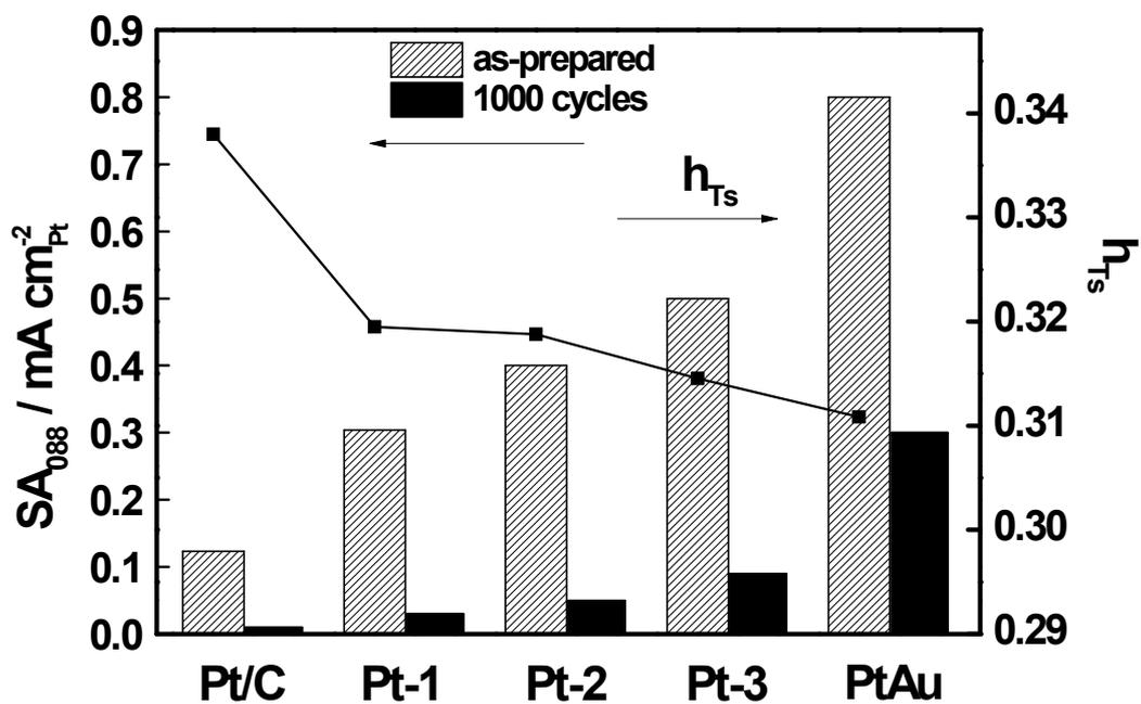
Figure S2 The comparisons of  $h_{\text{Ts}}$  and SA at 0.88 V before and after ADT for Pt/C and various NRs.
