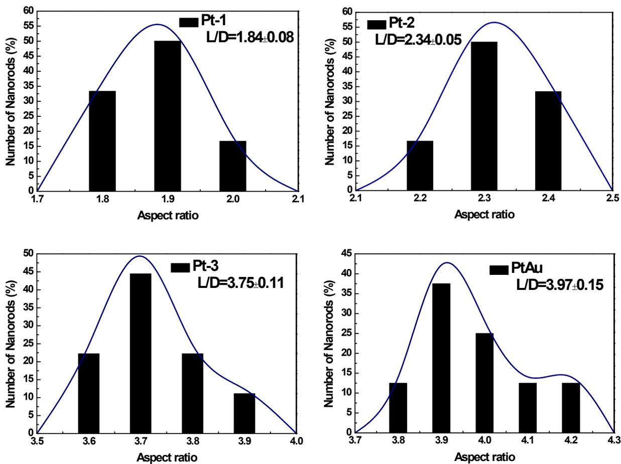
Figure S1 The aspect ratio distribution histograms of Pt-1, Pt-2, Pt-3, and PtAu NRs.
