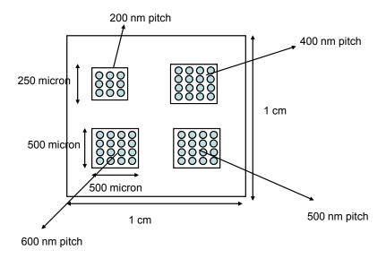
Fig.S1. Scheme of arrangement of the holes on the template. Hole diameter is 80 nm.
