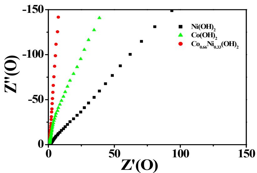
**Figure S5** Comparison of Nyquist plots of Ni-Co LDH hybrid-, nickel hydroxide-, and cobalt hydroxide- based electrodes.
