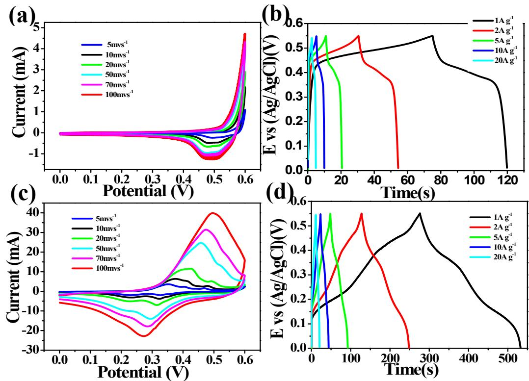
**Figure S4** CV curves obtained at different scan rates and galvanostatic charge-discharge curves obtained at different current densities for the sample pure  $\text{Ni}(\text{OH})_2$  (a,b) and pure  $\text{Co}(\text{OH})_2$  (c,d).
