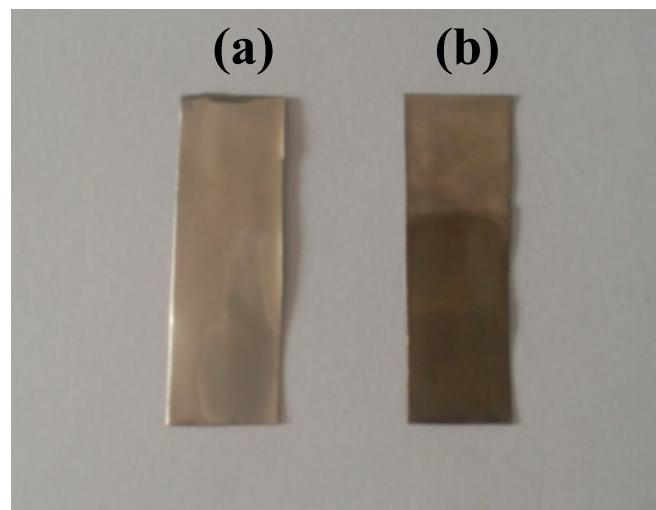
**Figure S1** Photograph of bare nickel sheet (a) and nickel-cobalt hydroxide nanosheets/nickel sheet (b) which used as working electrode.
