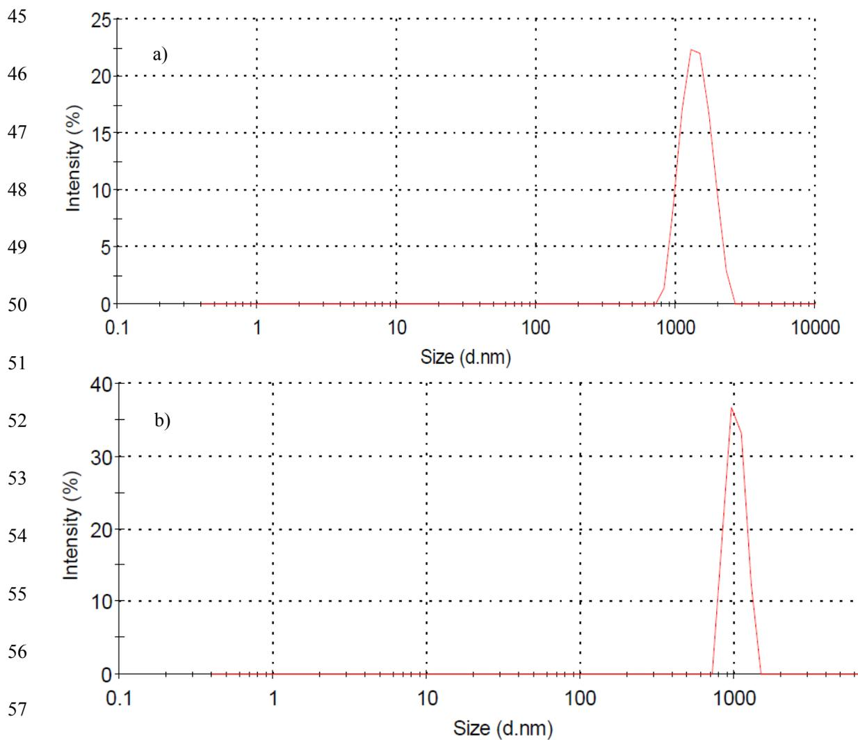
58 **Figure S2.** The particle size distribution curves of PCC 6803 (a), and TEB-PCC@UF (b).
