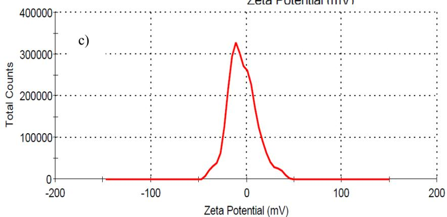
41 **Figure S1.** Zeta potential of the TEB-PCC spheres (a), UF prepolymers (b), and TEB-
