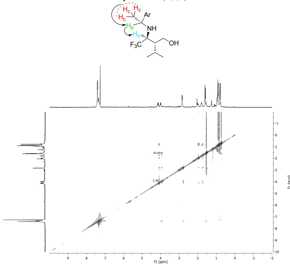
The cross peaks corresponding to the interproton correlations  $H_b/H_c$  (distance ruler setted to 10.00 au) and  $H_a/H_b$  (2.28 au), corresponding to an interproton distance of 3.44 Å, are evidenced. In Fig. 2 the interproton distance determined on the optimized geometries are reported.
