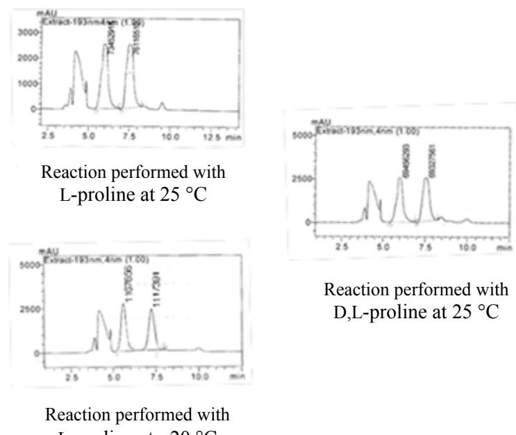
Chiralcel column; eluent: hexane/2-propanol = 95:5, flow 0.9 mL/min
