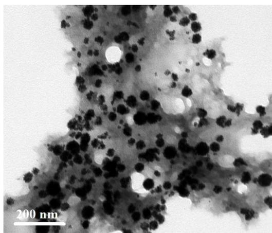
**Fig. S6** TEM images of the nanostructures produced by using CTAC as capping agents instead of Pluronic F127 in the typical synthesis.
