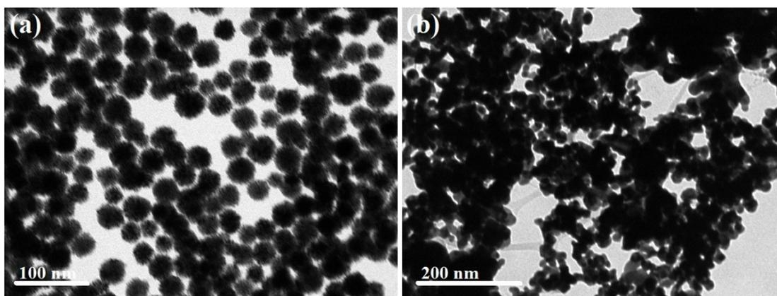
**Fig. S4** TEM images of the nanostructures produced by using (a) formic acid and (b)  $\text{NaBH}_4$  as reducing agents to replace ascorbic acid in the typical synthesis.
