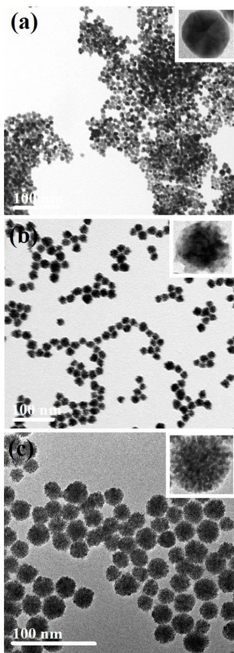
**Fig. S3** TEM images of the intermediate samples after (a) 10 seconds, (b) 5 minutes and (c) 10 minutes of reaction, respectively.
