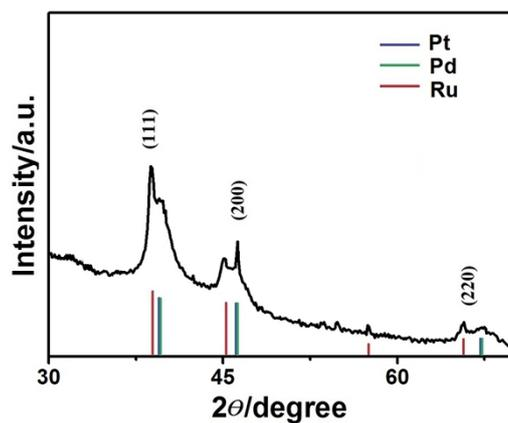
**Fig. S1** XRD pattern of the Pt-Pd-Ru nanodendrites. The positions of pure Pt, Pd and Ru at the bottom are taken from the JCPDS database.
