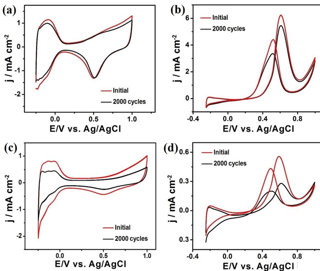
**Fig. S9** CVs for durability tests of Pt-Pd-Ru nanodendrites (a and b) and Pt/C (c and d) in 0.1 M  $\text{HClO}_4$  without (a and c) and with 1 M  $\text{CH}_3\text{OH}$  (b and d) at a scan rate of  $50 \text{ mV s}^{-1}$ . The current densities are normalized in reference to the geometric area of the working electrode.
