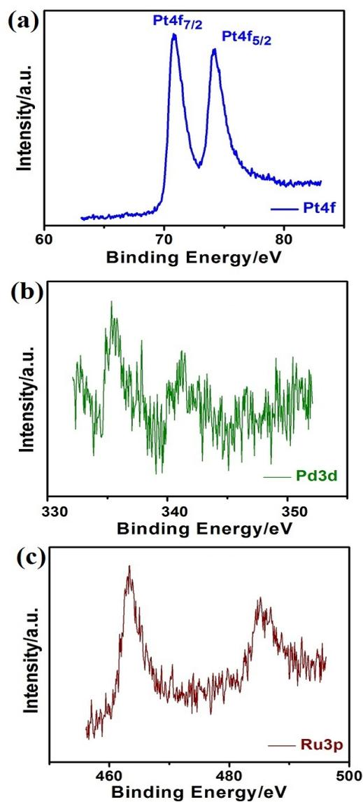
**Fig. S2** XPS spectra of the Pt-Pd-Ru nanodendrites centered on Pt *4f* (a), Pd *3d* (b) and Ru *3p* (c).
