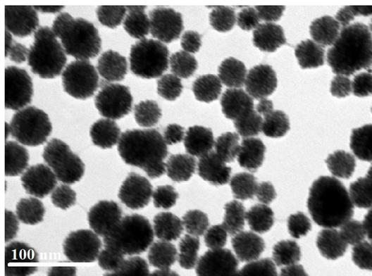
**Fig. S8** TEM image of the Pt-Pd-Ru nanodendrites prepared from 10 mM of Pt precursor.
