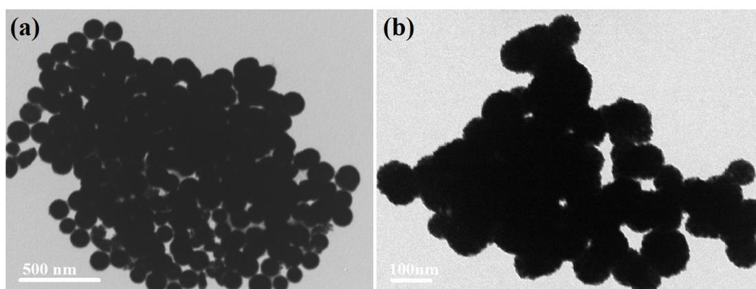
**Fig. S7** TEM images of the nanostructures synthesized without (a) and with (b) 0.001 g Pluronic F127, under the typical synthetic condition.
