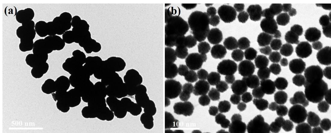
**Fig. S5** TEM images of the nanostructures synthesized by using of 0.1 M (a) and 0.2 M (b) AA, respectively, under the typical synthetic condition.
