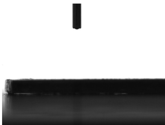
Fig. S7 The contact angle of water on the porous PPy nanostructure surface.
