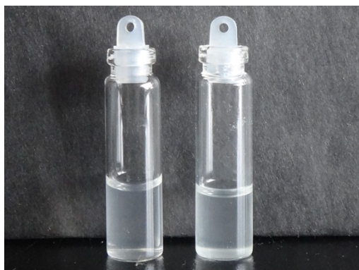
Figure S6. Dispersions of the \text{PW}_{12}\text{O}_{40}^{3-} based PIL Janus nanosheets in water (left) and toluene (right).
