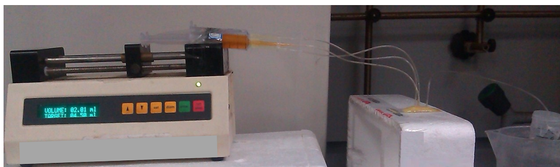
Fig. S2. Experimental setup for microfluidic synthesis of nanoplates. The left is the micro-pump; the middle is the micro-chip or reactor; the right is the collection of product in ice-water.
