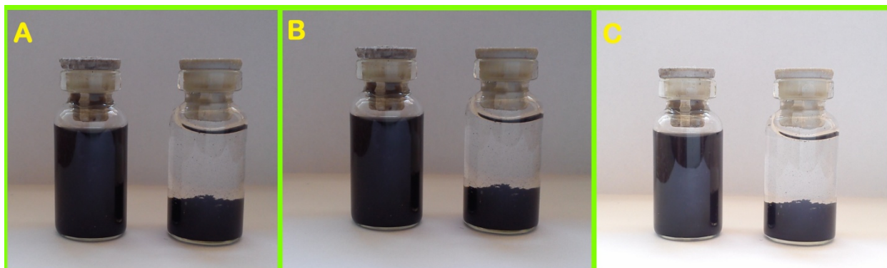
Figure S 1 . Photographs of TFPEG-treated MWCNT and pristine after (a) 12 h (b) 48 h (c) and 168 h
