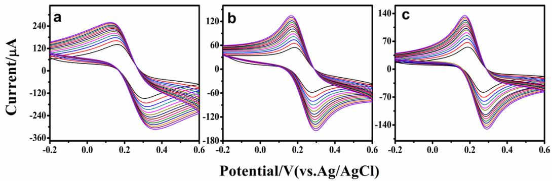
**Fig. S5** Cyclic voltammograms of 5 mM  $\text{K}_3[\text{Fe}(\text{CN})_6]/\text{K}_4[\text{Fe}(\text{CN})_6]$  in 0.1 M KCl at the bare CPE (a), GE (b), and GCE (c) at different scan rate. Scan rates: 20,30,40,50, 60,70,80,90,100,110,120, 130, 140, 150 mV  $\text{s}^{-1}$  (from bottom to top).
