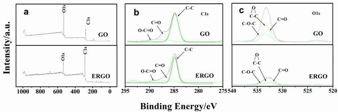
**Fig. S3** (a) Wide survey, (b) C 1s, and (c) O 1s XPS spectra of as-prepared GO (top) and ERGO (bottom) showing a significant reduction in the amount of oxygen containing functional groups on the ERGO from the reduction process.
