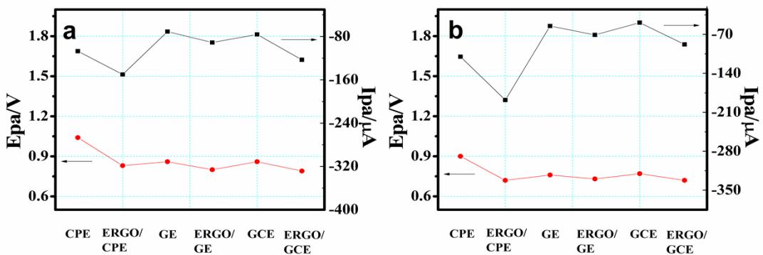
**Fig. S8** Peak potentials and currents of 5 mM  $\text{NaNO}_2$  containing in 0.2 M PBS (pH=7) at different bare and modified electrodes presented by CVs (a) and DPVs (b) (black and red curves for the bare electrode and ERGO modifieds, respectively).
