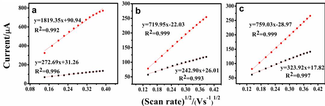
**Fig. S7** Plot of the peak currents of 5 mM  $\text{K}_3[\text{Fe}(\text{CN})_6]/\text{K}_4[\text{Fe}(\text{CN})_6]$  vs  $I^{1/2}$  for the CPE (a), GE (b), GCE (c) , respectively (black curves for the bare electrodes, red curves for the ERGO modified electrodes).
