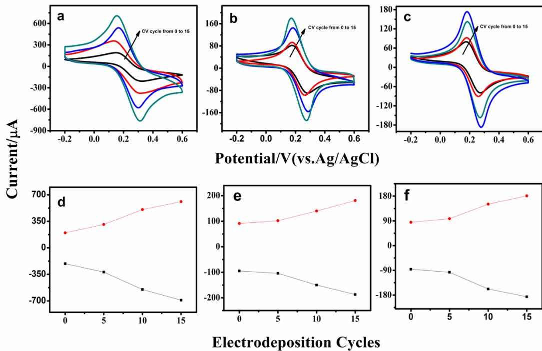
**Fig. S4** Cyclic voltammograms of 5 mM  $K_3[Fe(CN)_6]/K_4[Fe(CN)_6]$  in 0.1 M KCl at the as-prepared ERGO/CPE (a), ERGO/GE (b), ERGO/GCE (c) under different electrodeposition cycles of 0, 5, 10 and 15; Peak currents of 5 mM  $K_3[Fe(CN)_6]/K_4[Fe(CN)_6]$  in 0.1 M KCl at the as-prepared ERGO/CPE (a), ERGO/GE (b), ERGO/GCE (c) under different electrodeposition cycles.
