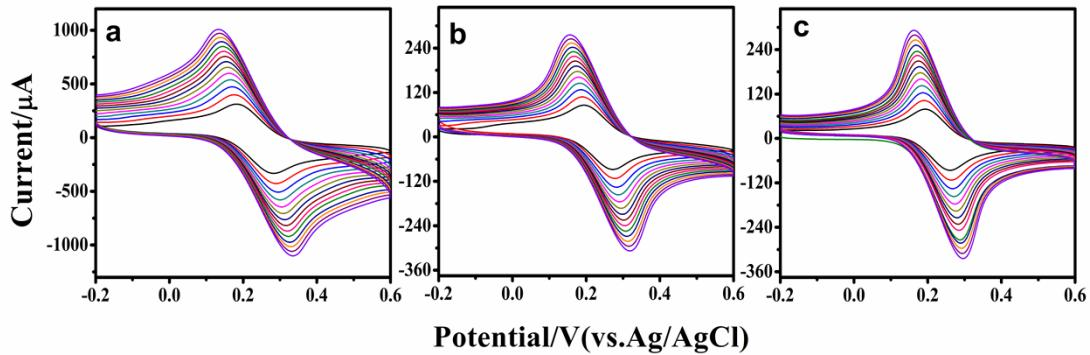
**Fig. S6** Cyclic voltammograms 5 mM  $\text{K}_3[\text{Fe}(\text{CN})_6]/\text{K}_4[\text{Fe}(\text{CN})_6]$  in 0.1 M KCl at the ERGO modified CPE (a), GE (b), and GCE (c) at different scan rate. Scan rates: 20,30,40,50, 60,70,80,90,100,110,120, 130, 140, 150 mV  $\text{s}^{-1}$  (from bottom to top).
