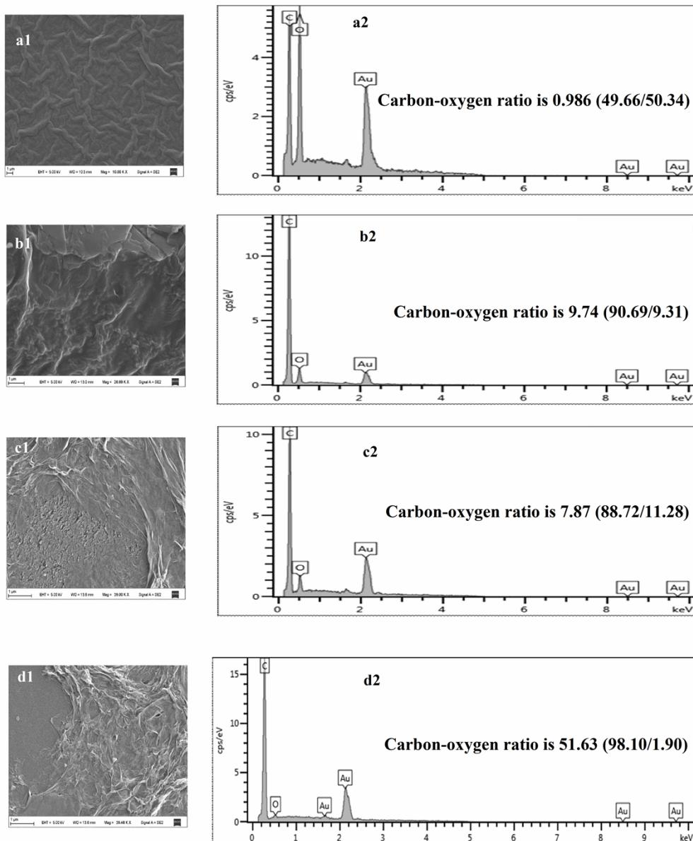
**Fig. S1** SEM and EDX of GO on GCE (a1, a2) and ERGO on CPE (b1, b2), GE (c1, c2), GCE (d1, d2).
