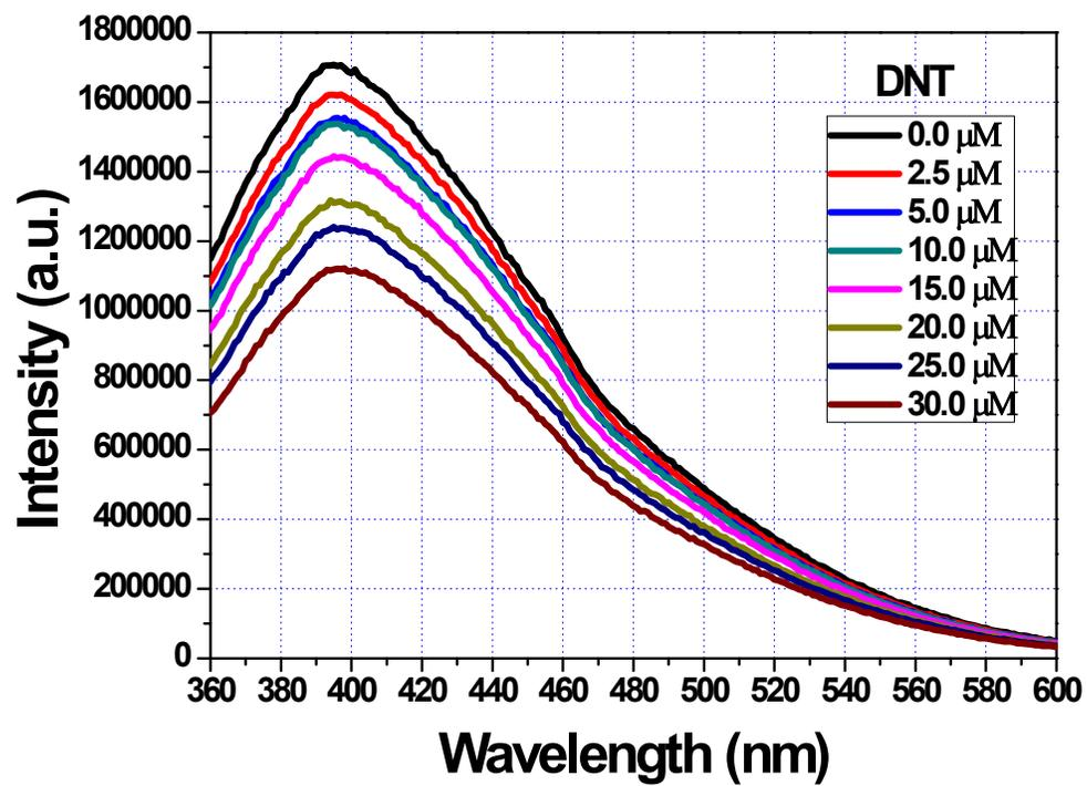
Fig. S8. Emission spectra of the composite solution upon incremental addition of acetonitrile solution of DNT ( $\lambda_{\text{ex}} = 314$  nm). Final concentration of DNT in the medium is indicated in the legend. All the spectra measured using Fluorolog Horiba Jobin-Yvon spectrofluorometer.
