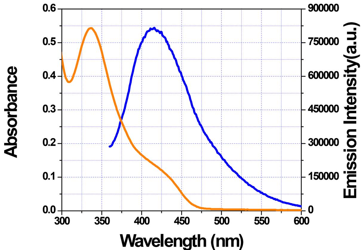
Fig. S22. Orange curve is absorption spectra of TNP in mixed solvent (acetonitrile and water in 1:2 volume ratio) (Conc. of analyte. = 50  $\mu$ M). Blue is the emission spectrum of composite solution which is nicely overlapped with the absorption band of TNP.
