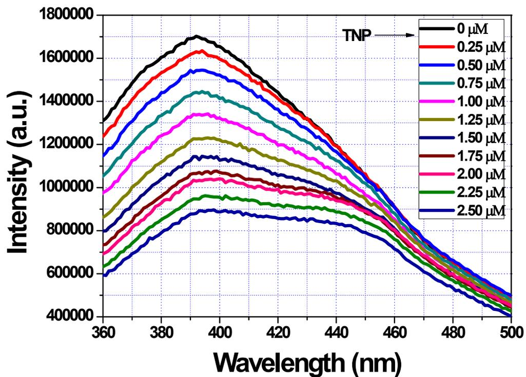
Fig. S4. Emission spectra of the composite solution upon incremental addition of acetonitrile solution of TNP ( $\lambda_{\text{ex}} = 314$  nm). Final concentration of TNP in the medium is indicated in the legend. All the spectra measured using Fluorolog Horiba Jobin-Yvon spectrofluorometer.
