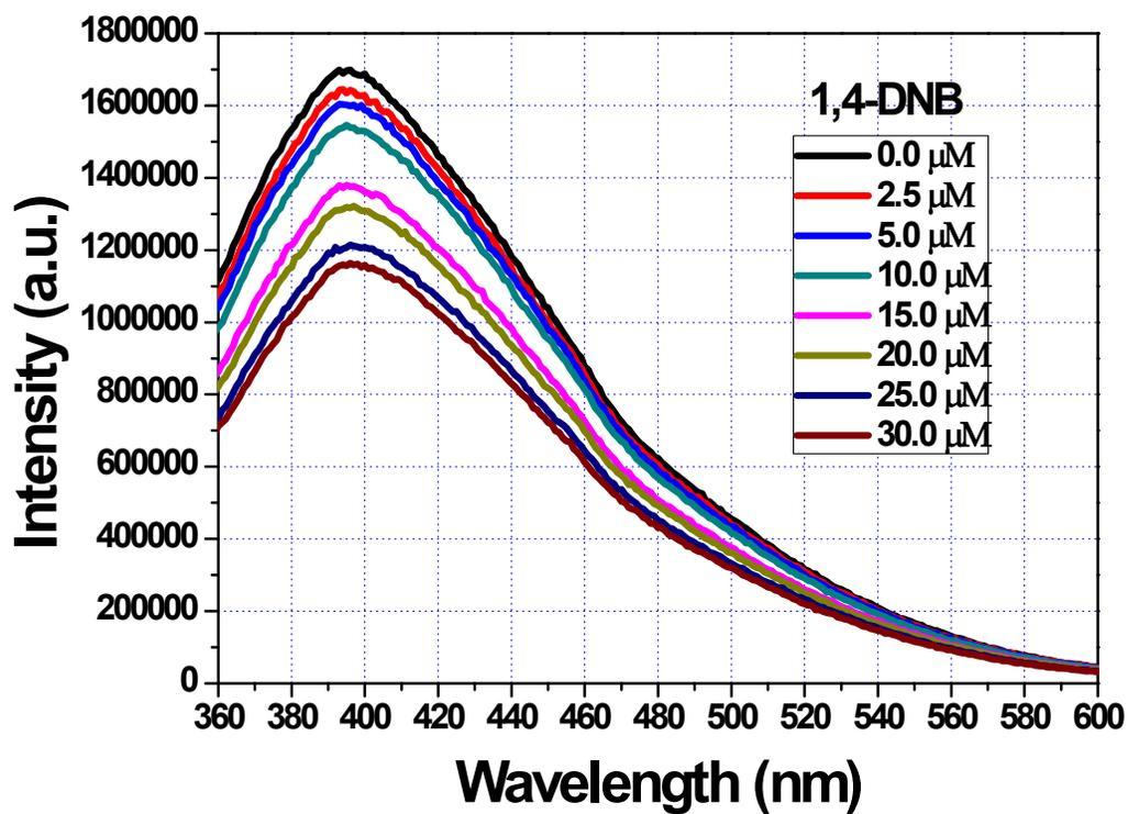
Fig. S7. Emission spectra of the composite solution upon incremental addition of acetonitrile solution of 1,4-DNB ( $\lambda_{\text{ex}} = 314 \text{ nm}$ ). Final concentration of 1,4-DNB in the medium is indicated in the legend. All the spectra measured using Fluorolog Horiba Jobin-Yvon spectrofluorometer.
