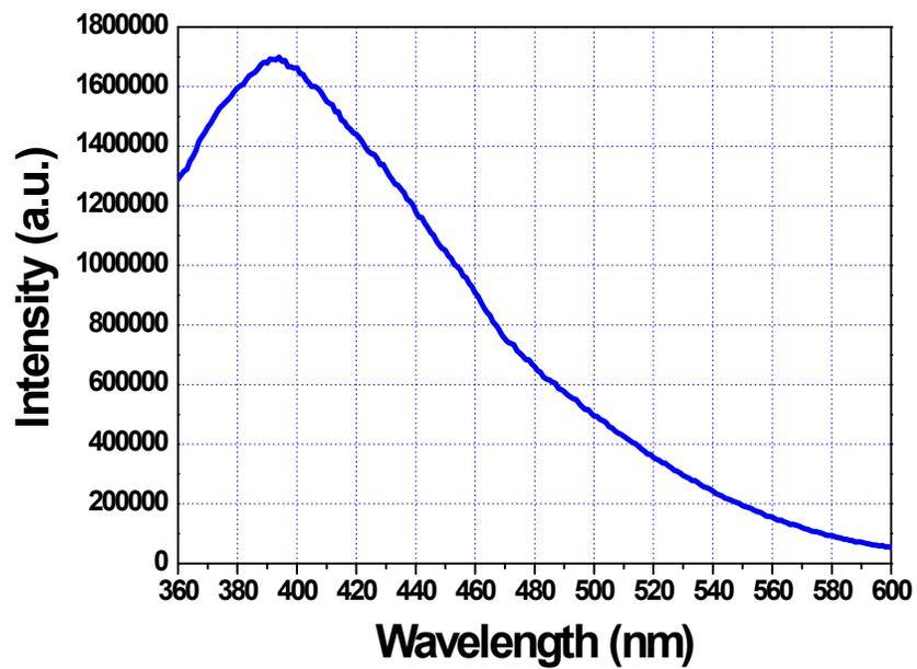
Fig. S2: Emission spectra of CP-C<sub>60</sub> composite solution ( $\lambda_{\text{ex}} = 314$  nm). Note the emission peak centered at 394 nm. The spectra measured using Fluorolog Horiba Jobin-Yvon spectrofluorometer.
