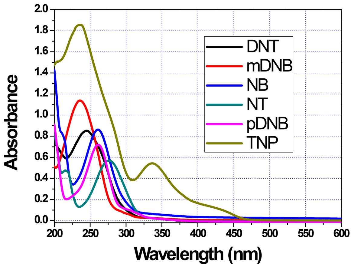
Fig. S21: Absorption spectra of all the six analytes in mixed solvent (acetonitrile and water in 1:2 volume ratio) (Conc. of analyte. = 50  $\mu$ M).
