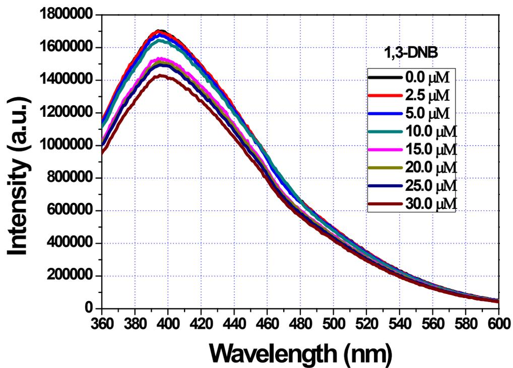
Fig. S6. Emission spectra of the composite solution upon incremental addition of acetonitrile solution of 1,3-DNB ( $\lambda_{\text{ex}} = 314$  nm). Final concentration of 1,3-DNB in the medium is indicated in the legend. All the spectra measured using Fluorolog Horiba Jobin-Yvon spectrofluorometer.
