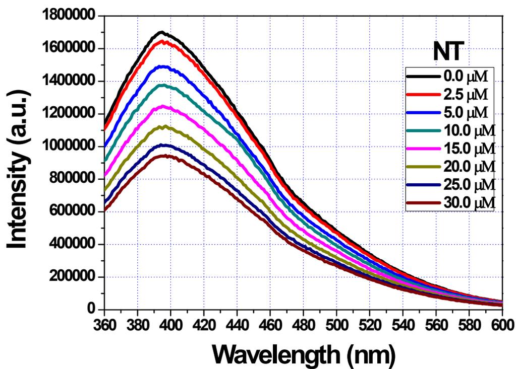
Fig. S9. Emission spectra of the composite solution upon incremental addition of acetonitrile solution of NT ( $\lambda_{\text{ex}} = 314$  nm). Final concentration of NT in the medium is indicated in the legend. All the spectra measured using Fluorolog Horiba Jobin-Yvon spectrofluorometer.
