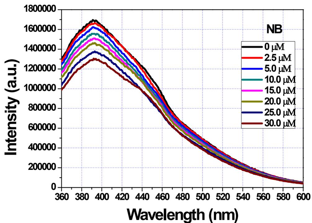
Fig. S10. Emission spectra of the composite solution upon incremental addition of acetonitrile solution of NB ( $\lambda_{\text{ex}} = 314$  nm). Final concentration of NB in the medium is indicated in the legend. All the spectra measured using Fluorolog Horiba Jobin-Yvon spectrofluorometer.
