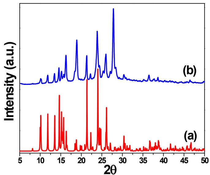
Fig. S1: Powder XRD ( $\text{CuK}\alpha$ ) patterns: (a) simulated from single crystal X-ray data of CP,  $[\text{Zn}(\text{L})_2(\text{H}_2\text{O})_2]$  ( $\text{L} = 3\text{-}(3\text{-pyridyl acrylate})$ ) [CCDC: 245503], (b) solvothermally synthesized CP (X. Li, R. Cao, Y. Sun, W. Bi, X. Li and Y. Wang, *Eur. J. Inorg. Chem.*, 2005, 321-329).
