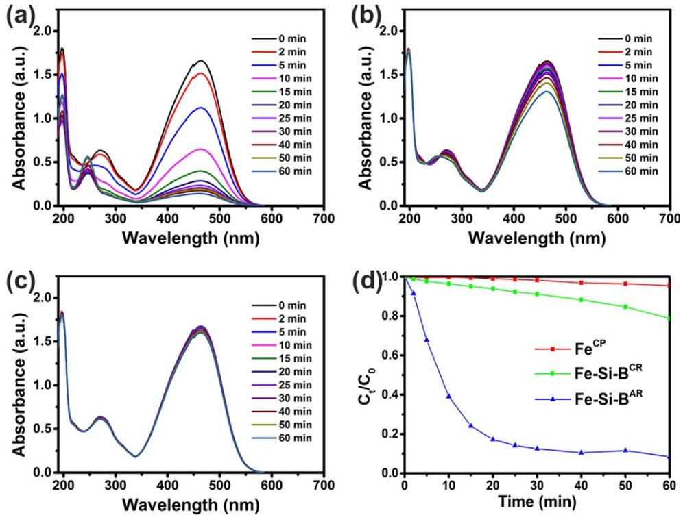
UV-vis spectroscopy ((a), (b), (c)) and normalized concentration (d) of Methyl Orange during the decomposition process: Uv-vis spectroscopy of different iron materials, (a) Fe-Si-B<sup>AR</sup>; (b) Fe-Si-B<sup>CR</sup>; (c) Fe<sup>CP</sup>. (Experimental conditions: 25 mg/L Methyl Orange, 10 g/L ribbons or powders, 25 °C, without addition any other reagents.)
