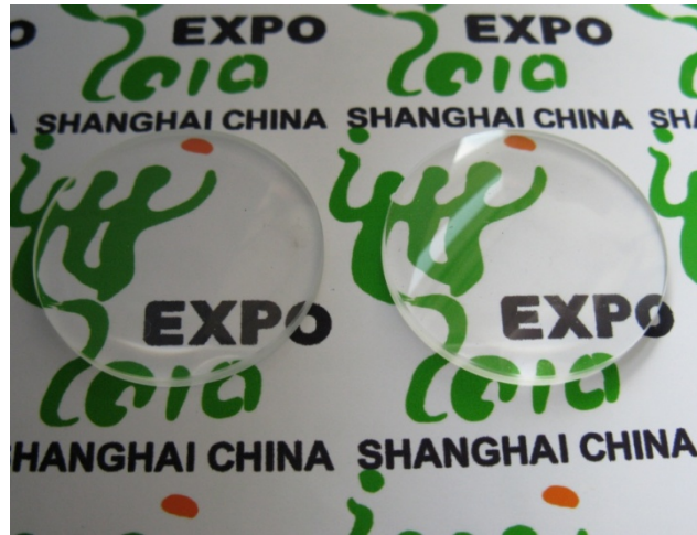
Figure S2. Photographs of the dual-sided structured lens (left) and planconvex lens (right).
