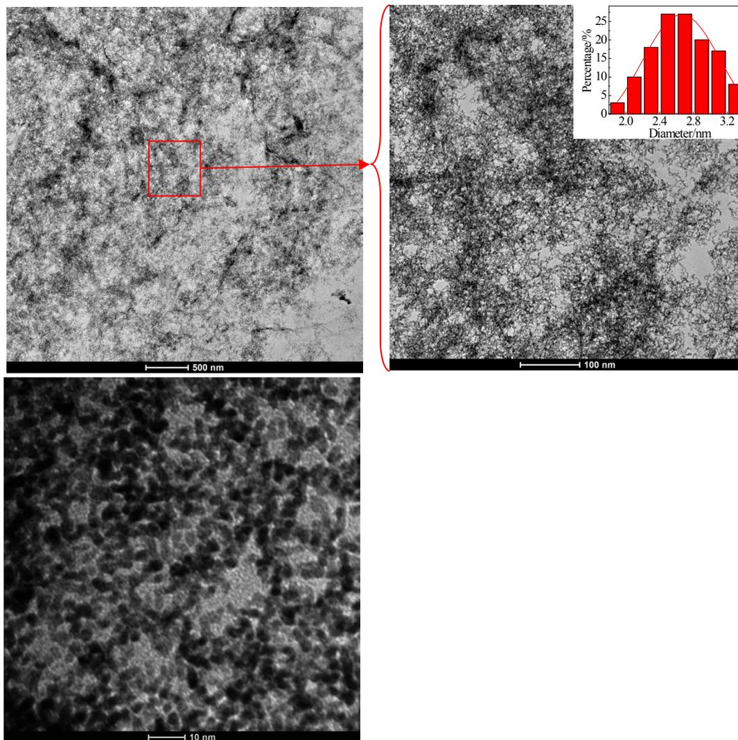
**Fig. S5.** TEM images of Pt<sub>52</sub>/RGO with different magnifications. The inset is the particle size distribution and the diameter is  $2.66 \pm 0.02$  nm.
