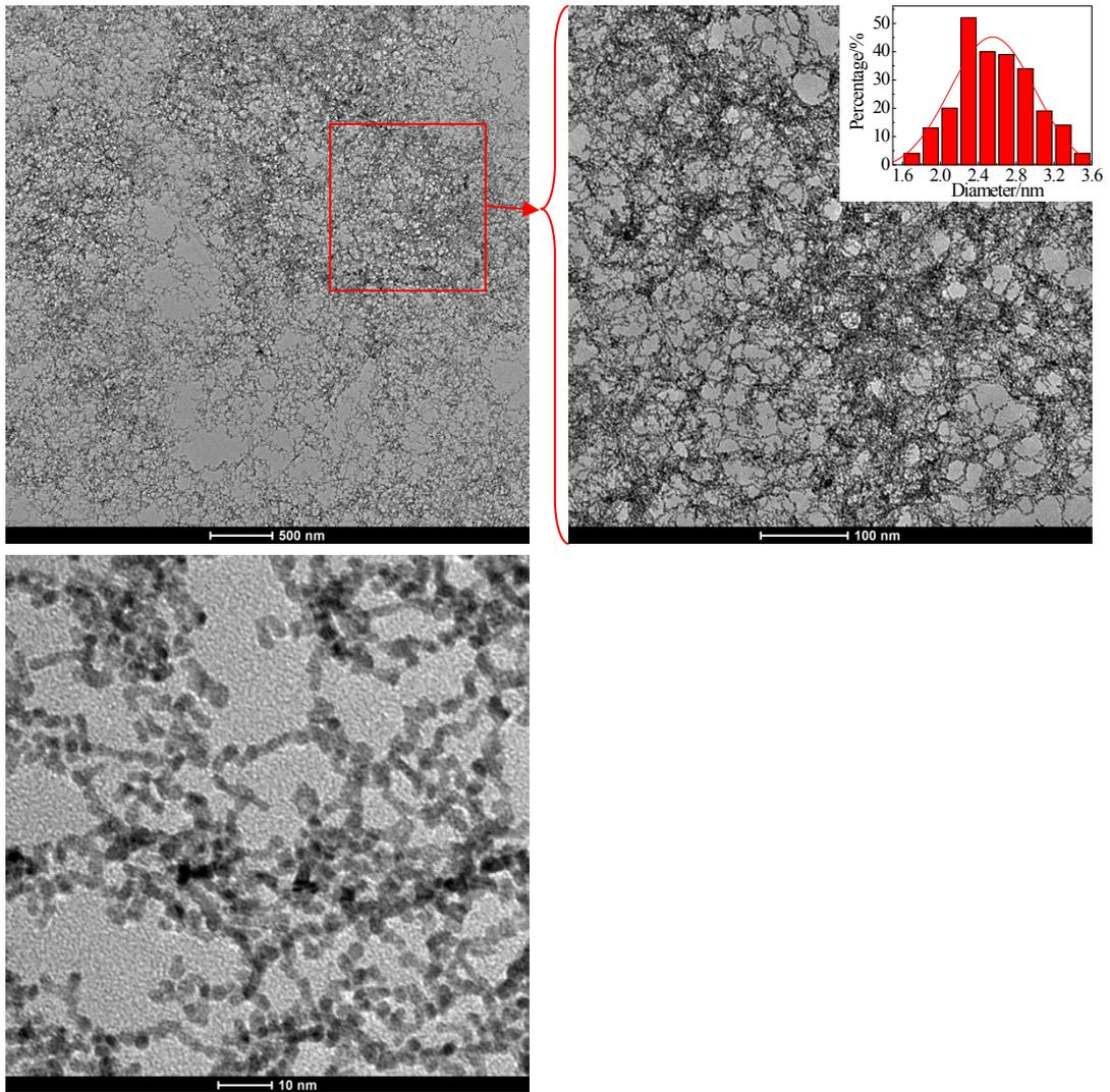
**Fig. S4.** TEM images of Pt<sub>39</sub>/RGO with different magnifications. The inset is the particle size distribution and the diameter is  $2.55 \pm 0.04$  nm.
