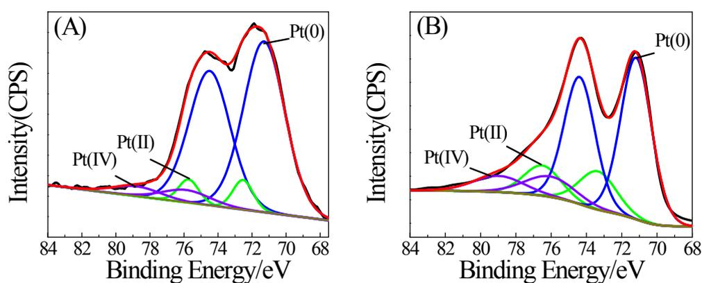
**Fig. S1.** Pt4f XPS spectra of Pt nanoparticles and the commercial Pt/C catalyst. Black curves are the original patterns; red curves are the simulated patterns by the curves of the deconvoluted components marked in each figure.
