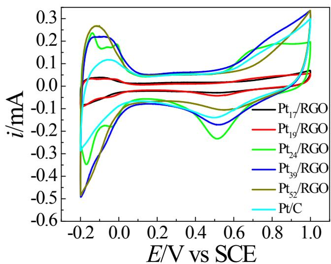
**Fig. S6.** Cycle voltammograms of five Pt/RGO composites and the commercial Pt/C in 0.5 mol/L  $\text{H}_2\text{SO}_4$  at a scan rate of  $50 \text{ mV}\cdot\text{s}^{-1}$ .
