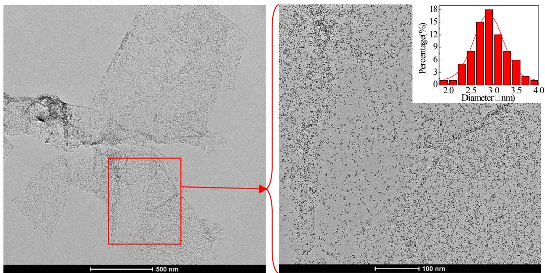
**Fig. S2.** TEM images of Pt<sub>17</sub>/RGO with different magnifications. The inset is the particle size distribution and the diameter is  $2.88 \pm 0.02$  nm.
