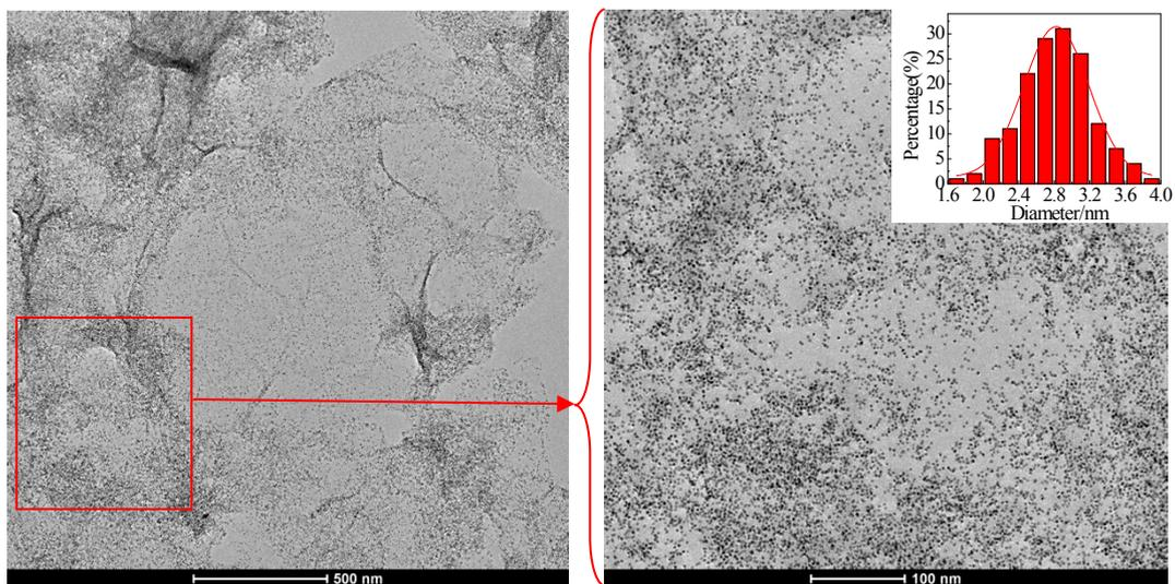
**Fig. S3.** TEM images of Pt<sub>19</sub>/RGO with different magnifications. The inset is the particle size distribution and the diameter is  $2.82 \pm 0.02$  nm.
