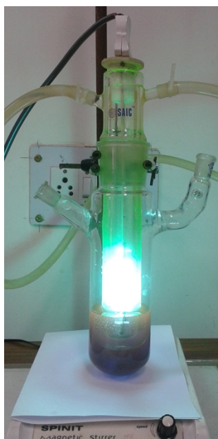
Figure S2: Setup for dye degradation
