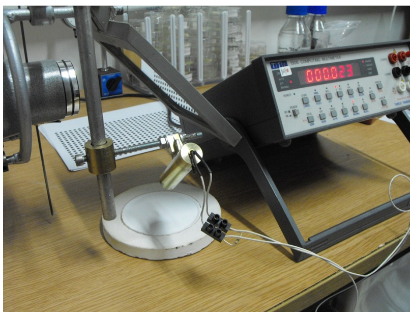
Figure S1. Diffuse ( 0^\circ/45^\circ ) reflectance measurement. The barium sulphate disc is shown.
