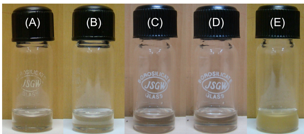
Figure S7: Digital photographs of Cho-Gly after dissolution of DNA in different concentrations (A) 2 wt %, (B) 4 wt %, (C) 6 wt %, (D) 8 wt %, and (E) 10 wt %.
